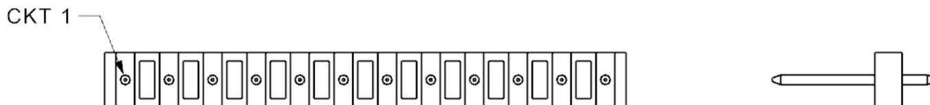
**10.3 PCB Headers with Polarizing Backwall (Series: [2599](#))**
