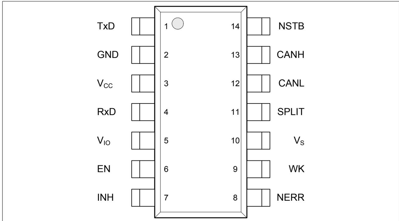
Figure 2 Pin Configuration
