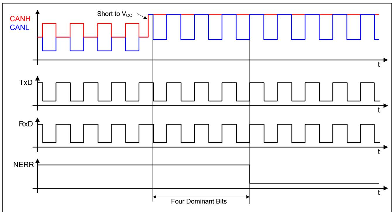
**Figure 9 CAN Bus Failure CANH short to  $V_{CC}$**
