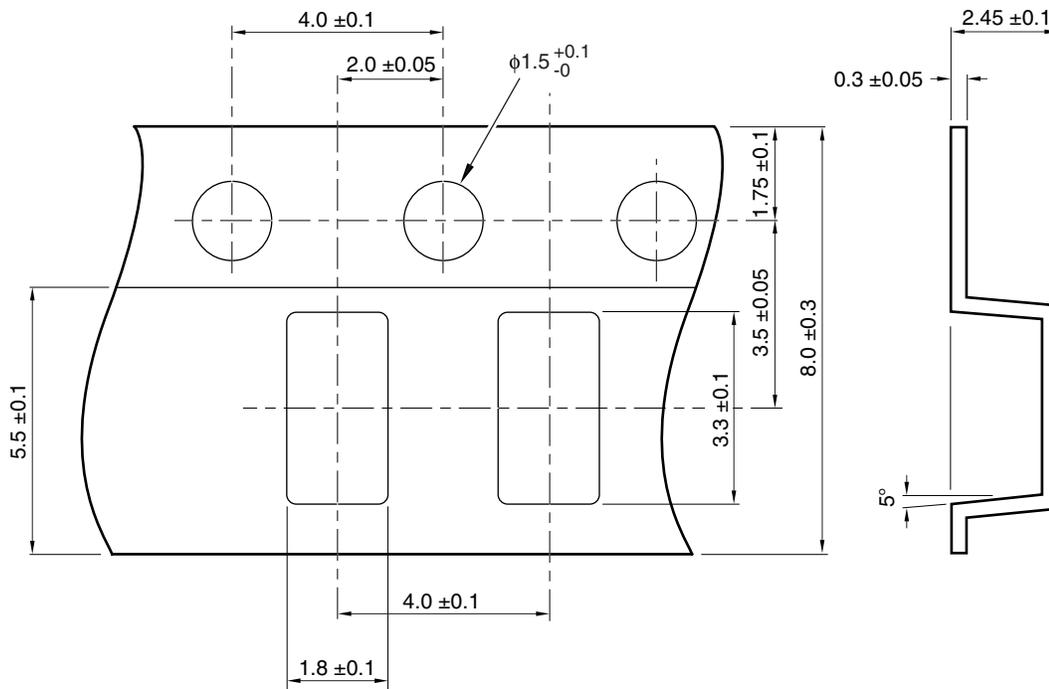
Fig. 15 Reel Shape and Dimension
