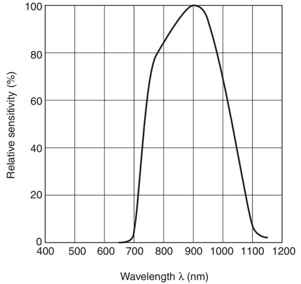
**Fig. 7 Radiation Diagram (TYP.)**
