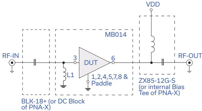
Fig 1. Application and Characterization Circuit
