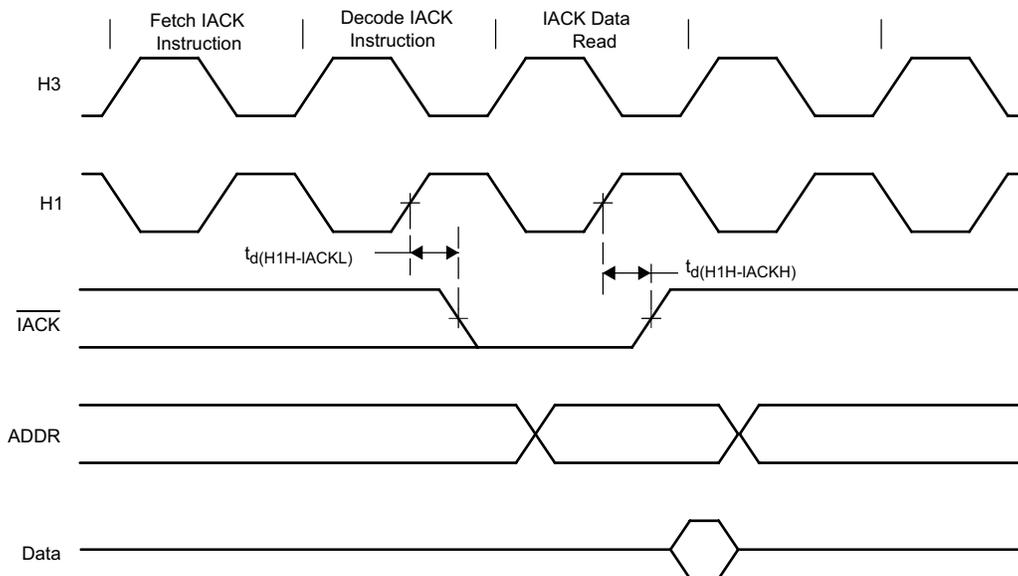
Figure 16. Interrupt Acknowledge ( $\overline{IACK}$ ) Timing
