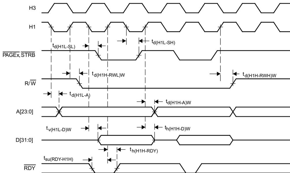
Figure 7. Timing for Memory (STRB = 0 and PAGEx = 0) Write
