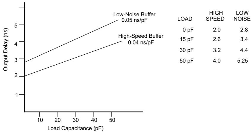
This figure shows output load characteristics for high-speed and low-speed (low-noise) output buffers. High-speed buffers are used on A0 to A23, PAGE0 to PAGE3, H1, H3, STRB, and R/W. All other outputs use the low-speed, (low-noise) output buffer.
