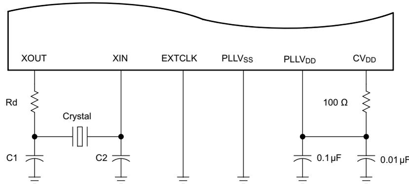
**Figure 26. Self-Oscillation Mode**
