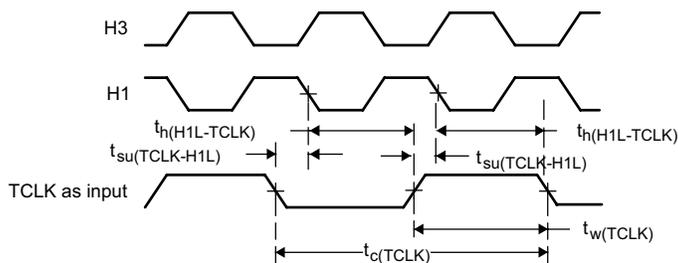
Figure 21. Timer Pin Timing, Input
