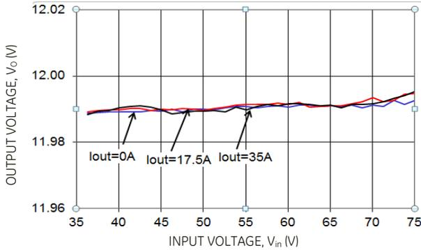
Figure 7. Typical Output Voltage Regulation vs. Input Voltage.
