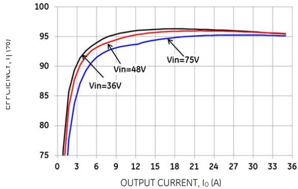
Figure 2. Typical Converter Efficiency vs. Output Current.
