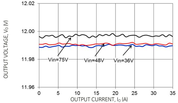
Figure 8. Typical Output Voltage Regulation vs. Output Current.
