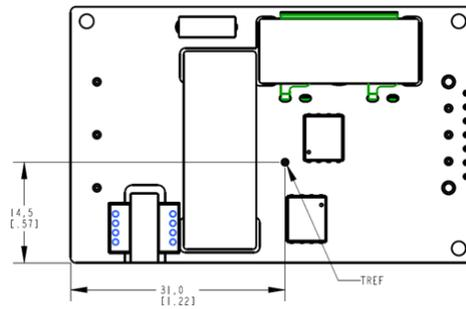
Figure 16. Location of the thermal reference temperature TH.
