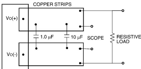
Note: Use a 1.0 μF ceramic capacitor and a 10 μF aluminum or tantalum capacitor. Scope measurement should be made using a BNC socket. Position the load between 51 mm and 76 mm (2 in. and 3 in.) from the module.
