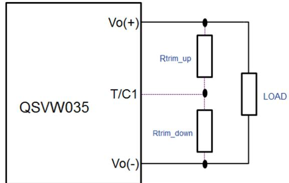
Figure 15. Circuit Configuration to Trim Output Voltage.
