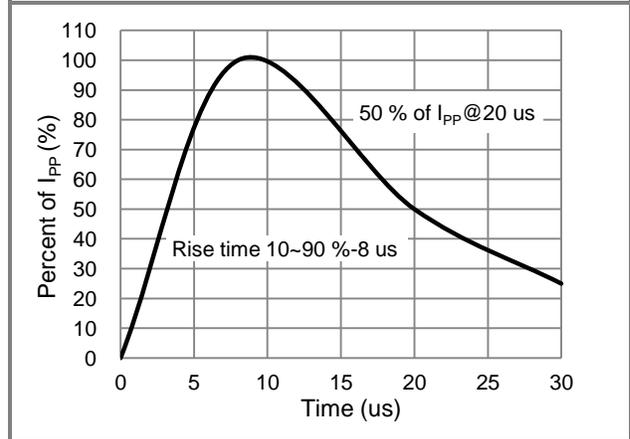
Fig.2 Pulse Waveform
