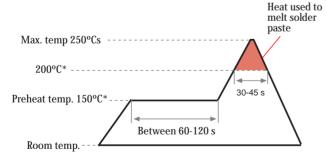
\* Melting point temp. depends on solder properties
