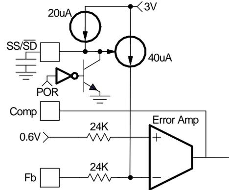
Fig. 5: Soft-Start circuit for IR3822A
