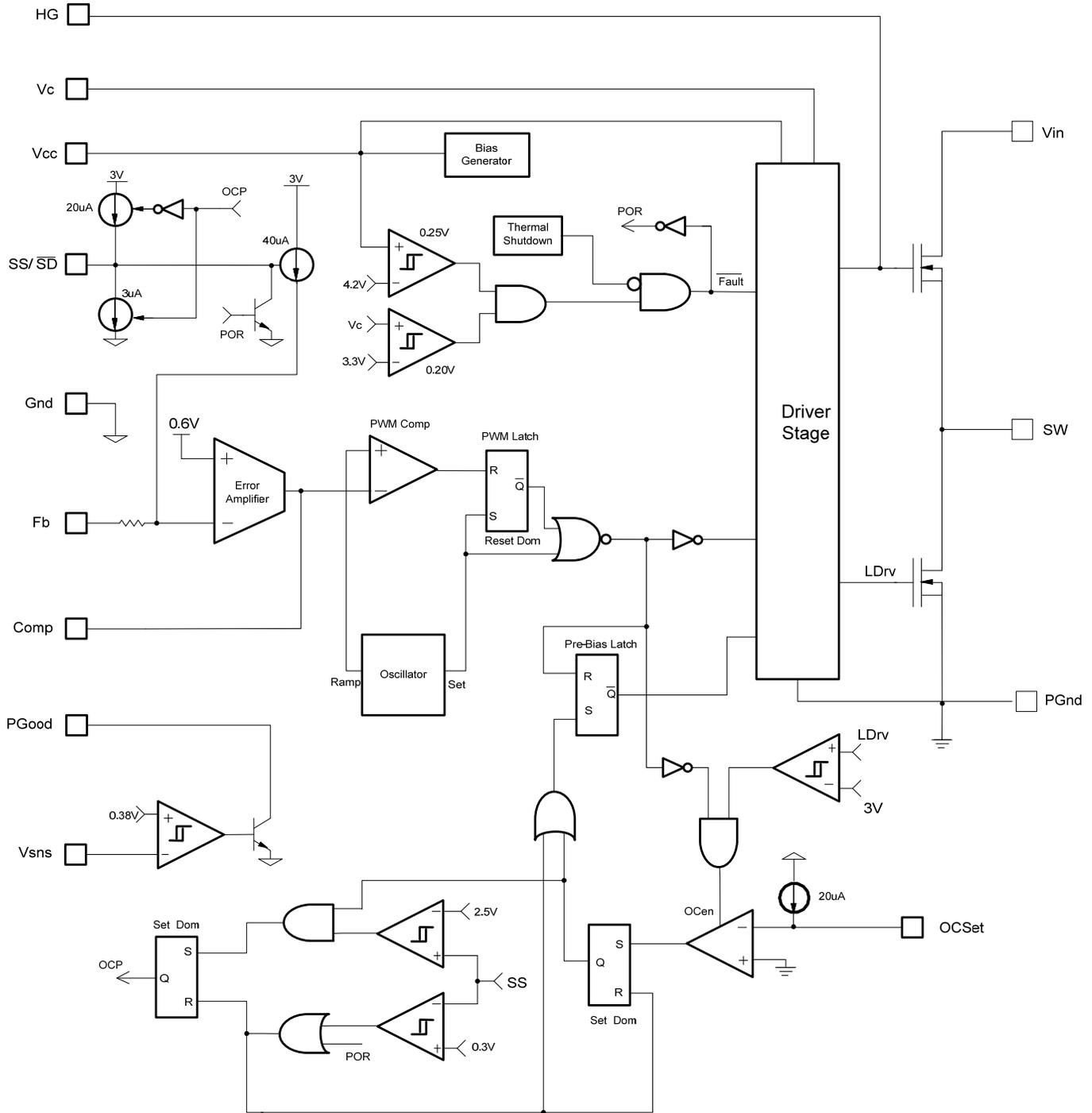
Fig. 3. Simplified block diagram of the IR3822A.
