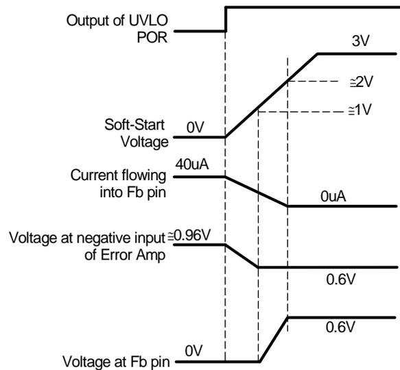
Fig. 6: Theoretical operation waveforms during soft-start
