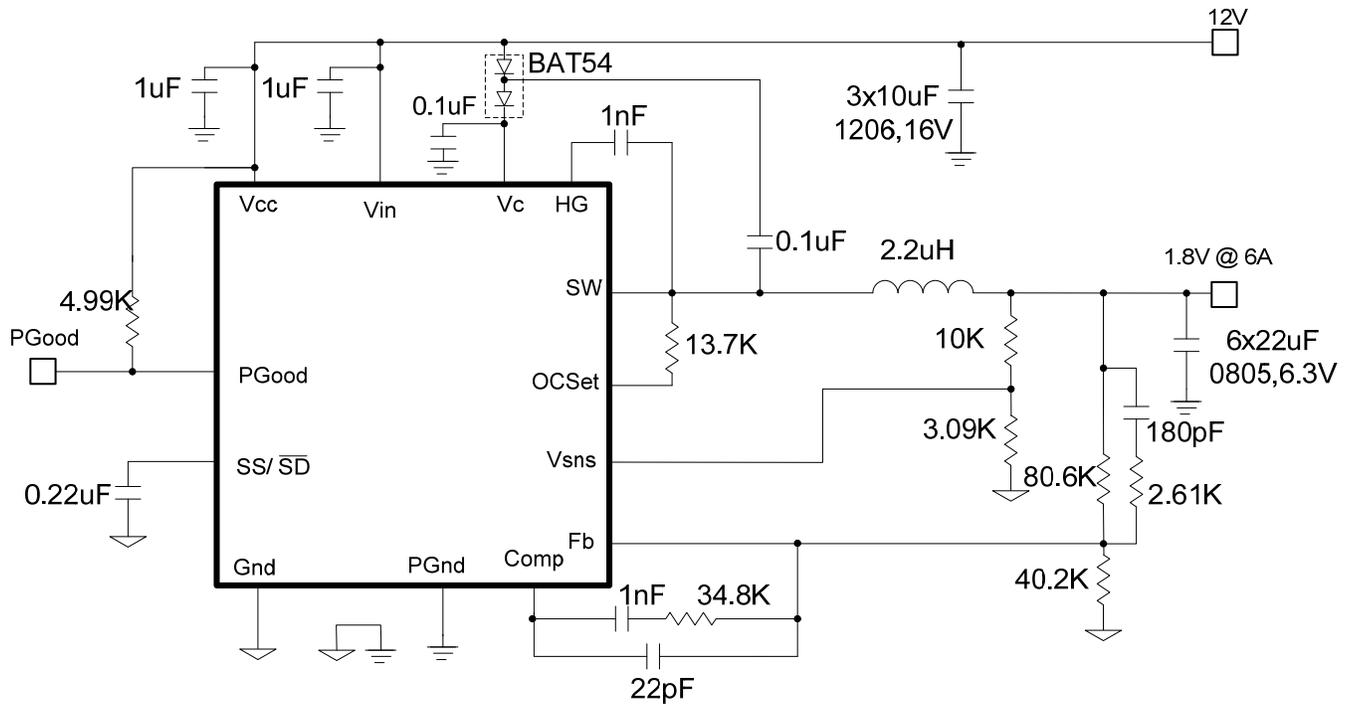
Fig.16: Typical Application circuit for 12V to 1.8V at 6A using ceramic output capacitors
