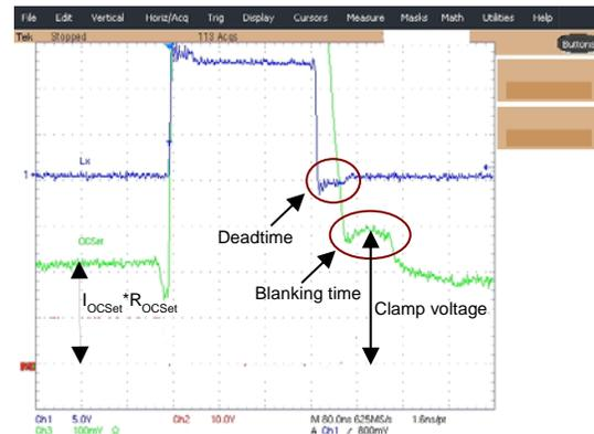
Fig. 9: OCset pin during normal condition
