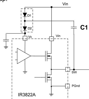
Fig. 11: Charge pump circuit to generate  $V_c$  voltage
