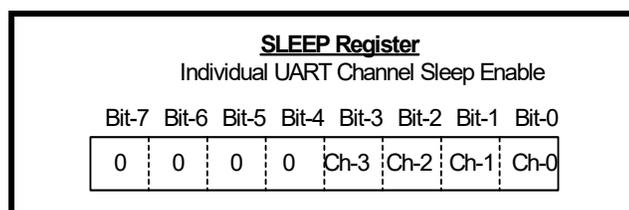
The 8-bit SLEEP register enables each UART separately to enter Sleep mode. The SLEEP register is accessible from the Device Configuration Registers in all UART channels but the UART channel can only control the bit for that channel. For example, writing 0xFF to the SLEEP register in channel 0 will only enable the sleep mode for channel 0.
