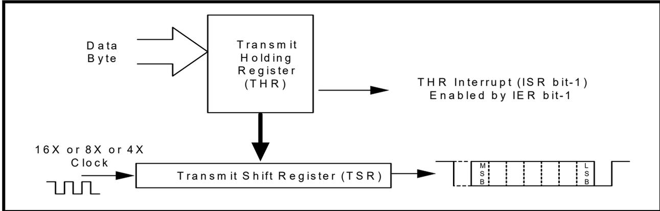
**3.6.3 Transmitter Operation in FIFO Mode**
