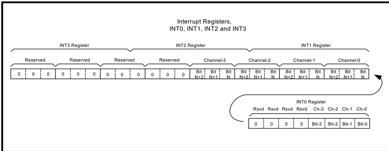
TABLE 7: UART CHANNEL [3:0] INTERRUPT SOURCE ENCODING
