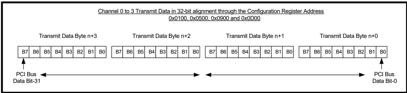
**2.2 FIFO DATA LOADING AND UNLOADING THROUGH THE UART CHANNEL REGISTERS, THR AND RHR IN 8-BIT FORMAT**
