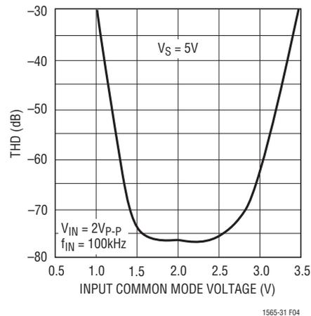
Figure 4. THD vs Common Mode Input Voltage
