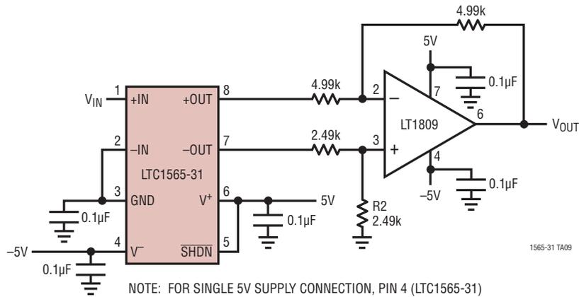
NOTE: FOR SINGLE 5V SUPPLY CONNECTION, PIN 4 (LTC1565-31) AND PIN 4 (LT1809) SHOULD BE GROUNDED AND RESISTOR R2 SHOULD BE DC BIASED AT APPROXIMATELY 2.5V (SEE TEST CIRCUIT FOR SINGLE SUPPLY OPERATION)
