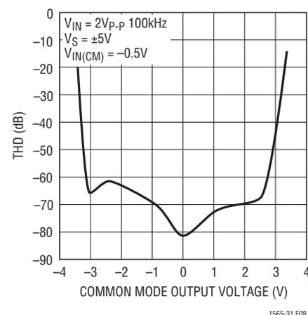
Figure 8. THD vs Common Mode Output Voltage
