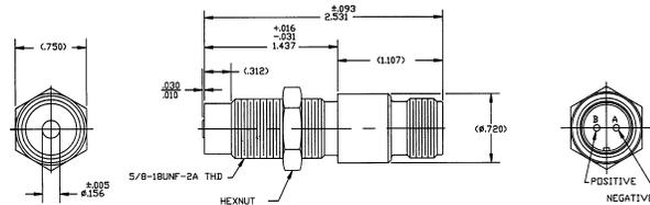
SENSORS WITH 5/8-18 UNF-2A MOUNTING THREAD\*, 1/2-14
