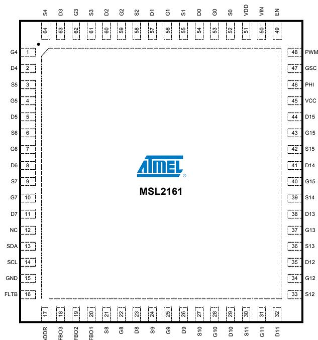
**Figure 1. Atmel LED Driver-MSL2161 Pin-out, 64-pin TQFN.**
