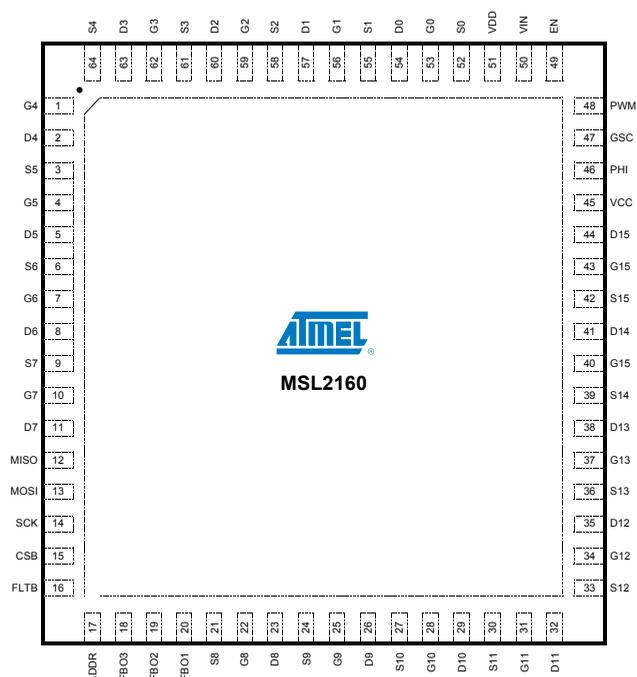
**Figure 2. Atmel LED Driver-MSL2160 Pin-out, 64-pin TQFN.**
