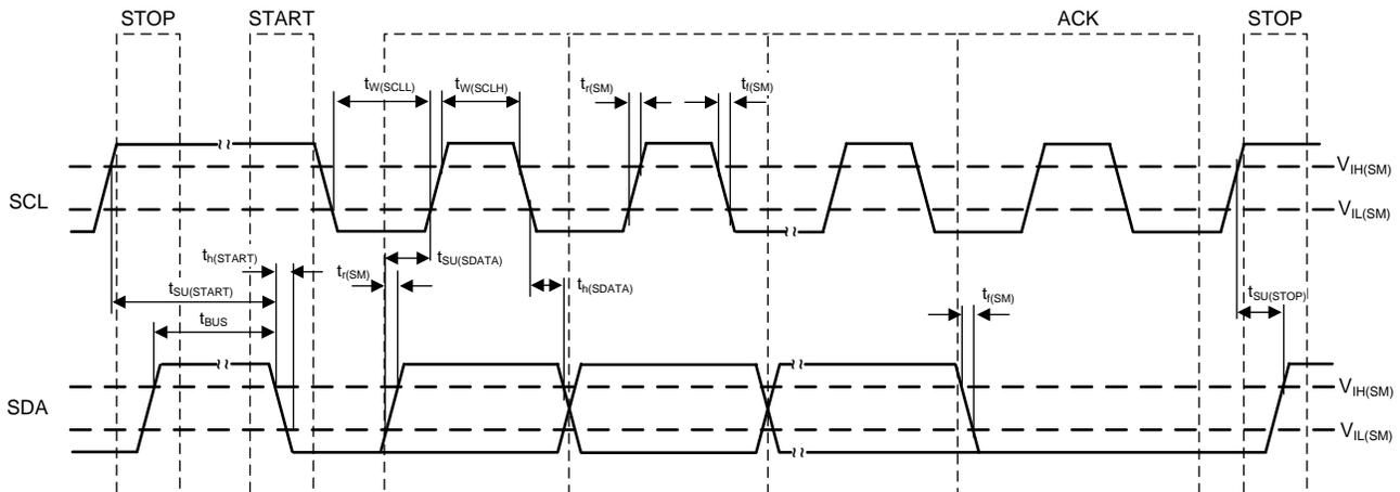
**Figure 8. I<sup>2</sup>C Timing Diagram**
