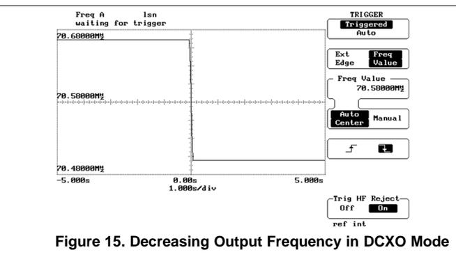
Figure 15. Decreasing Output Frequency in DCXO Mode
