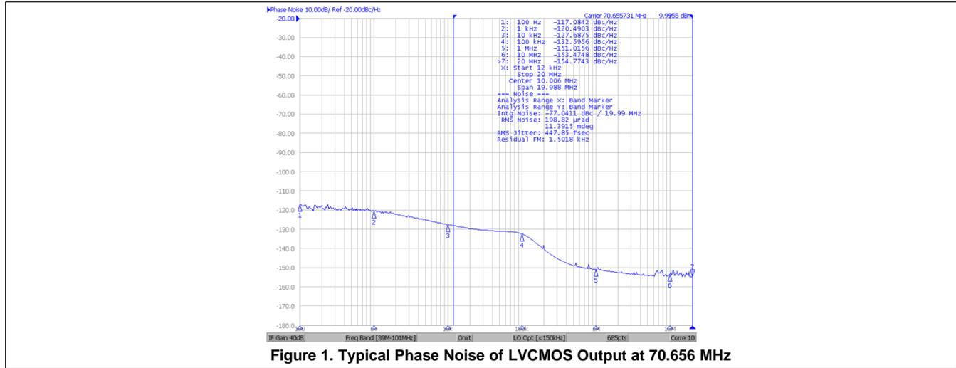
Figure 1. Typical Phase Noise of LVCOS Output at 70.656 MHz
