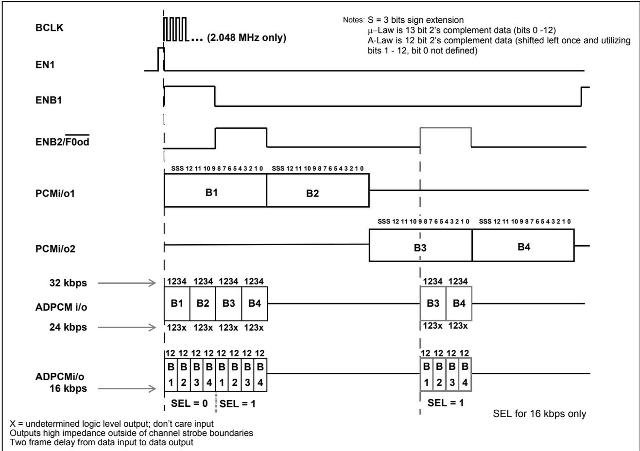
Figure 5 - SSI 16-Bit Linear PCM Relative Timing
