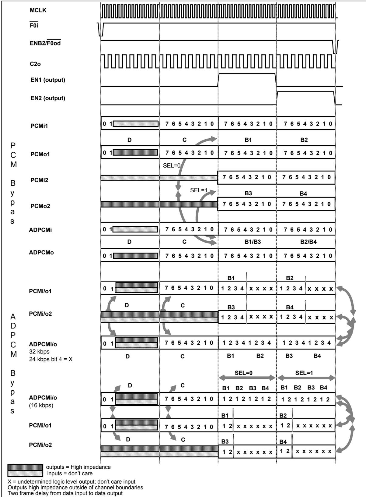
Figure 9 - ST-BUS PCM and ADPCM Bypass Relative Timing
