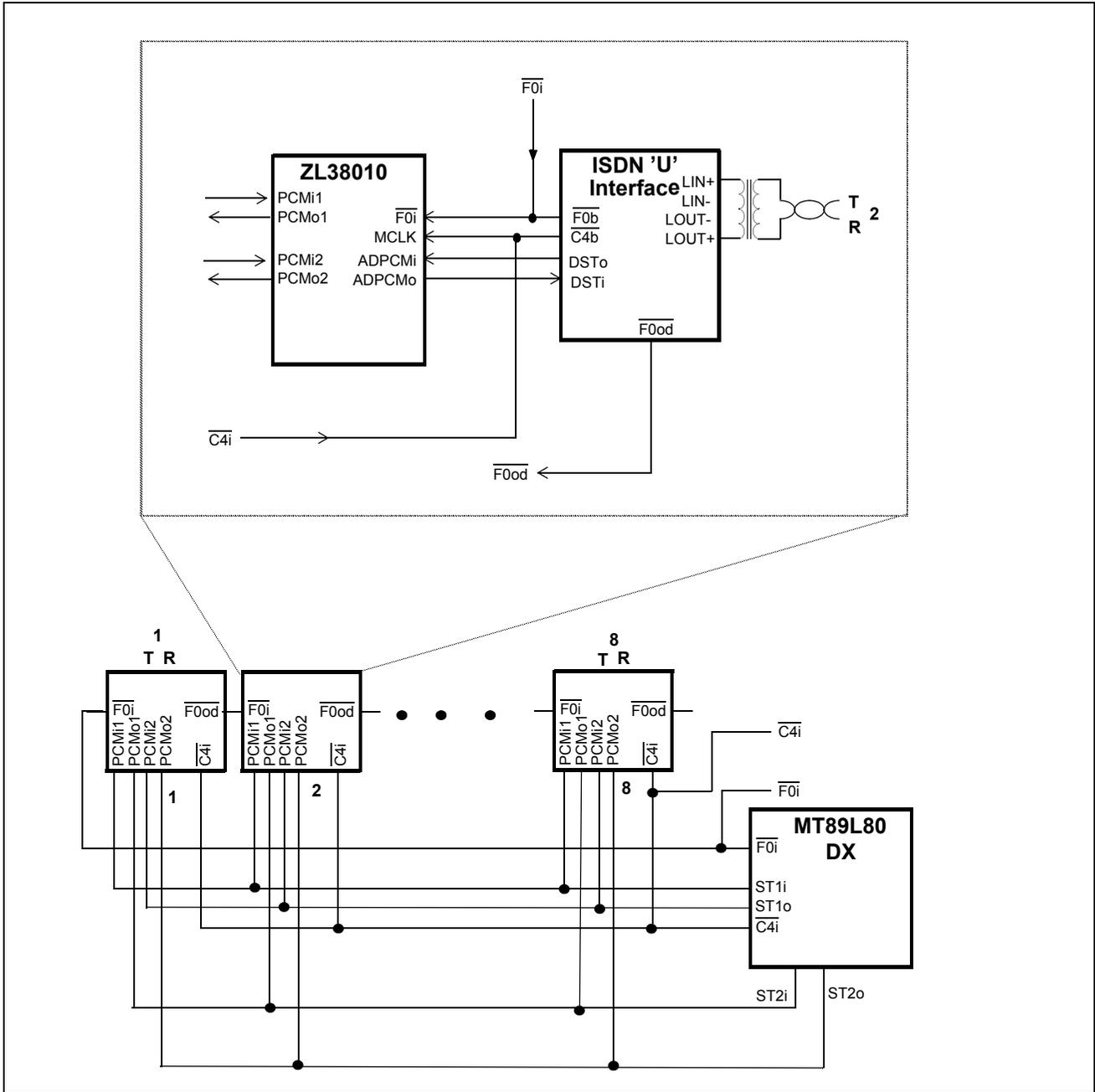
Figure 11 - ISDN Line Card with 32 kbps ADPCM
