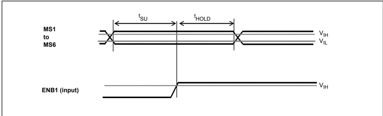
**Figure 16 - SSI Mode Select Set-up and Hold Timing**
