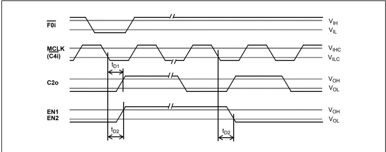
**Figure 15 - ST-BUS Timing for External Signal Generation**
