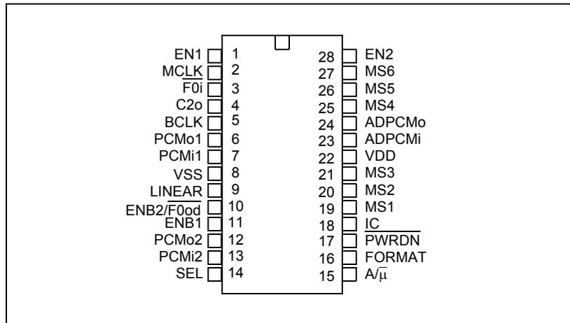
Figure 2 - Pin Connections
