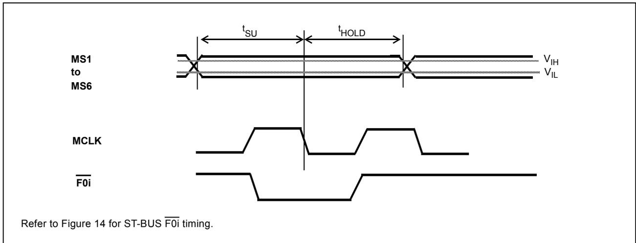
**Figure 17 - ST-BUS Mode Select Set-up and Hold Timing**
