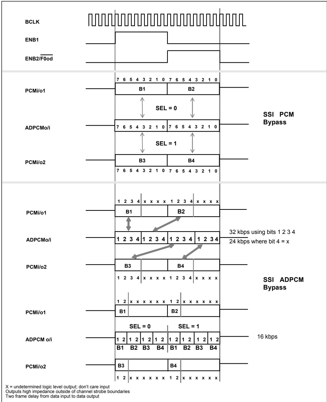
Figure 6 - SSI PCM and ADPCM Bypass Relative Timing
