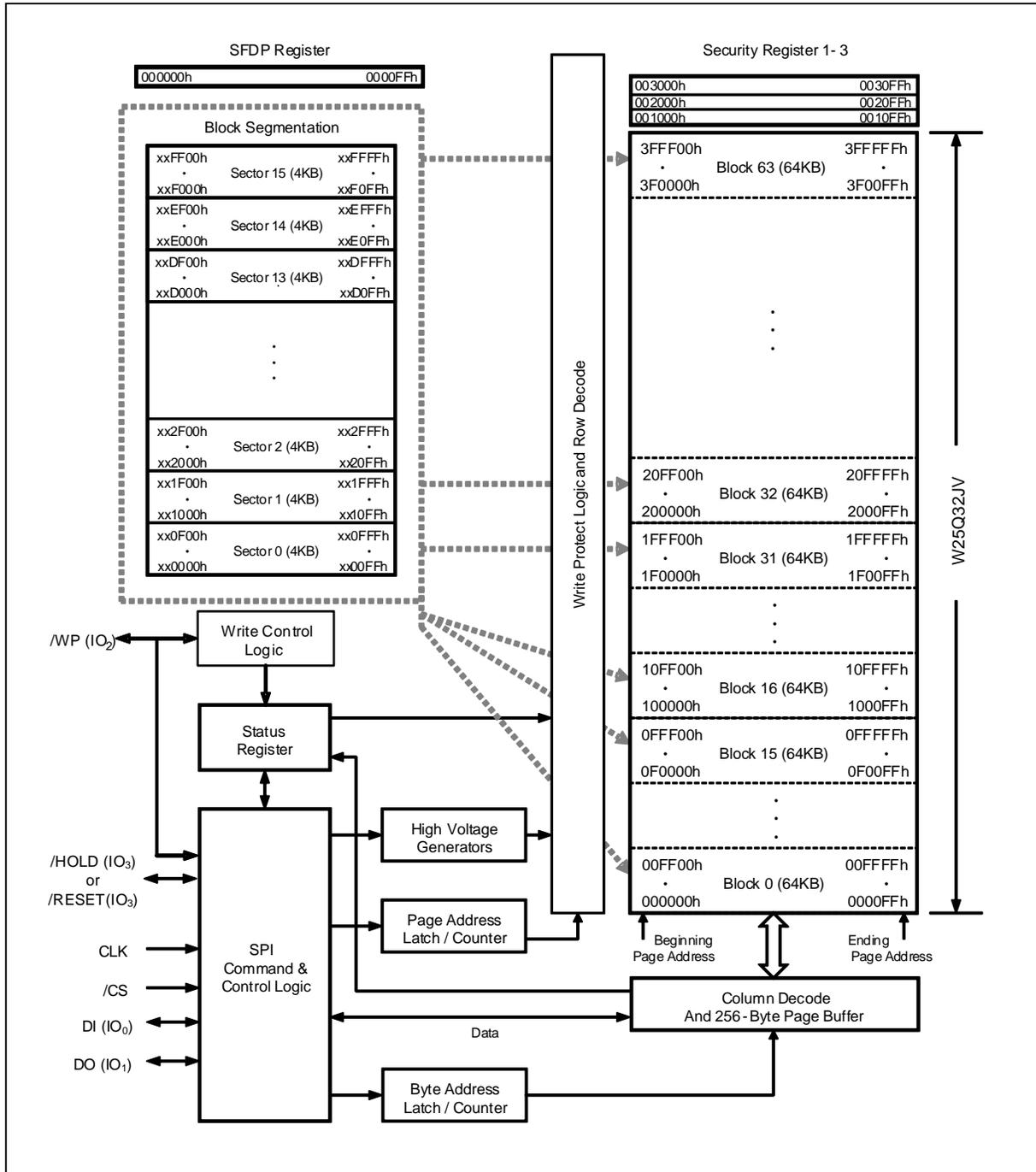
Figure 2. W25Q32JV Serial Flash Memory Block Diagram
