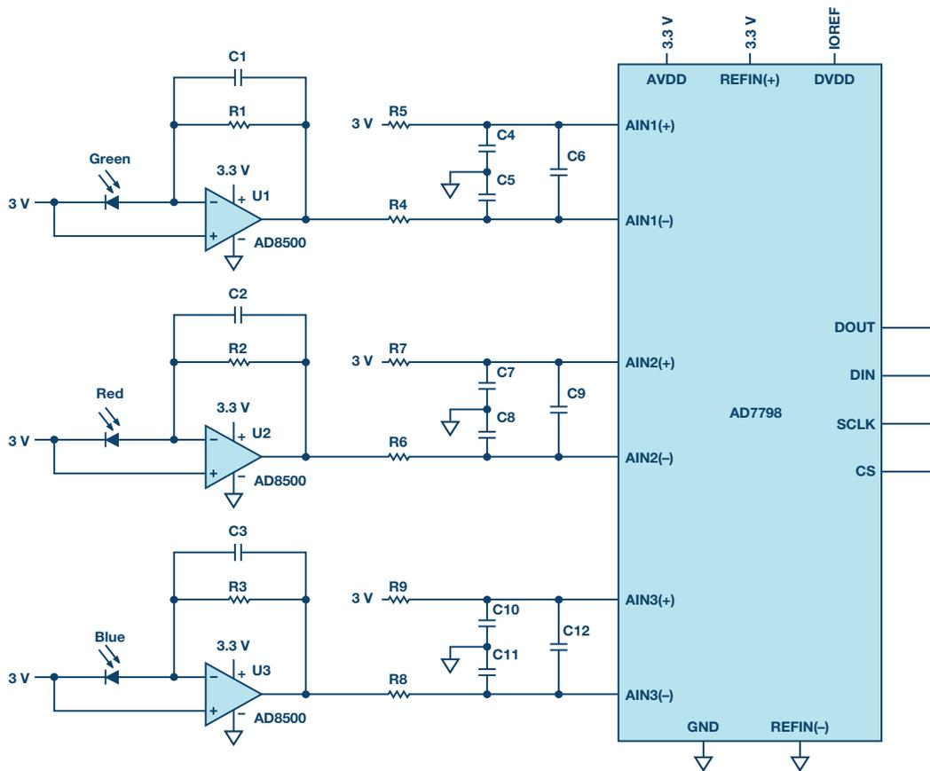
Figure 1. Circuit design for measurement of light intensity.
