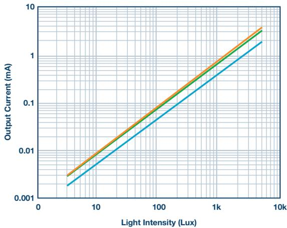
Figure 2. Characteristic curves of current to light intensity for red, green, and blue photodiodes.
