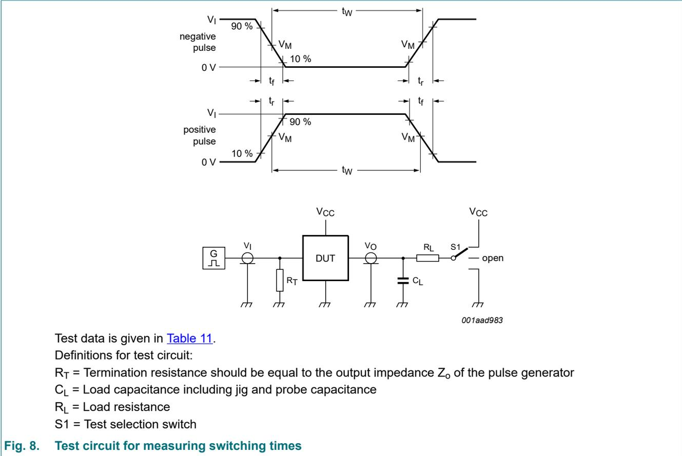
**Fig. 8. Test circuit for measuring switching times**
