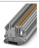
Knife disconnect terminal block, with actuation latch, Connection type: Screw connection, Cross section: 0.14 mm² - 6 mm², AWG: 26 - 10, Nominal current: 20 A, Nominal voltage: 500 V, Length: 57.8 mm, Width: 6.2 mm, Color: gray, Assembly: NS 35/7,5, NS 35/15
