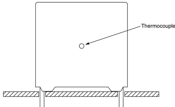
The temperature is measured in unloaded ( $T_{\text{amb}}$ ) and maximum loaded condition ( $T_{\text{C}}$ ).
