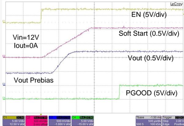
Figure 20. Startup Waveforms with Pre-Bias Voltage on Output
