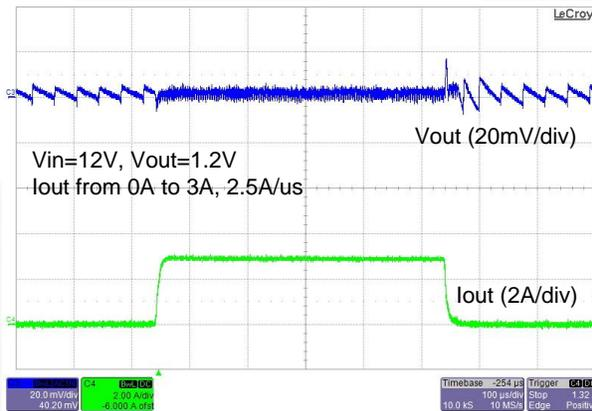
Figure 25. FAN2306A Load Transient from 0% to 50% Load Current
