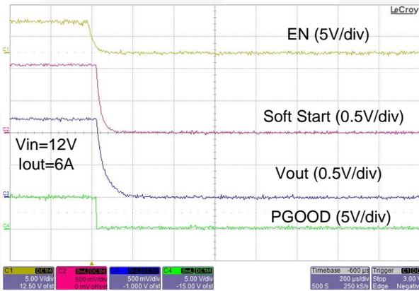
Figure 19. Shutdown Waveforms with 6 A Load Current
