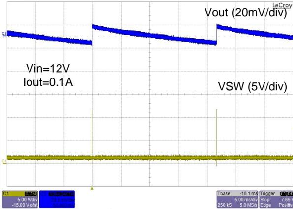
Figure 13. FAN2306MA Static Output Ripple with No Load
