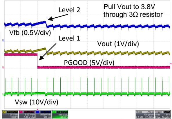
Figure 29. Over-Voltage Protection Level 1 and Level 2
