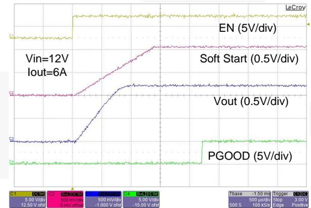
Figure 16. Startup Waveforms with 6 A Load Current
