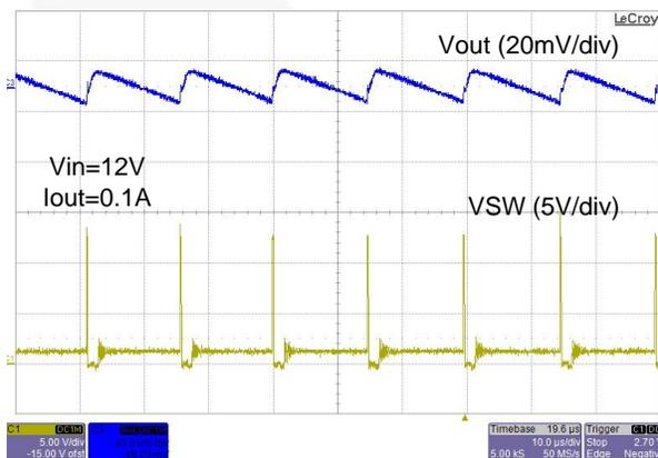
Figure 21. FAN2306A Static Output Ripple at Light Load
