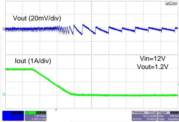
Figure 24. FAN2306A Transition from CCM to DCM
