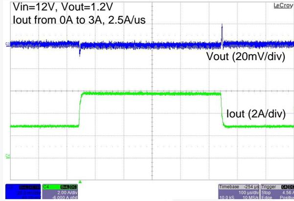
Figure 26. Load Transient from 50% to 100% Load Current
