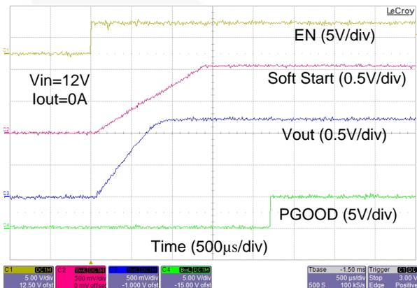
Figure 15. Startup Waveforms with 0 A Load Current
