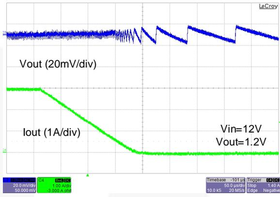
Figure 18. FAN2306MA Transition from CCM to DCM
