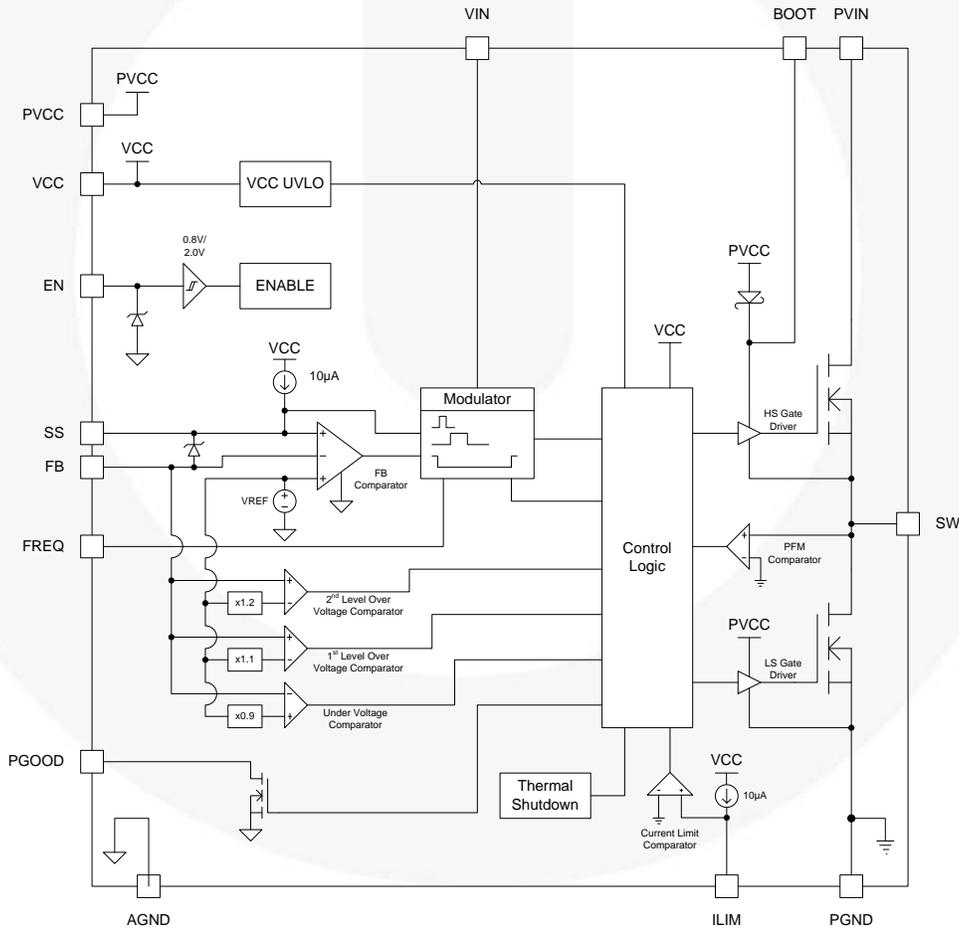
Figure 2. Block Diagram
