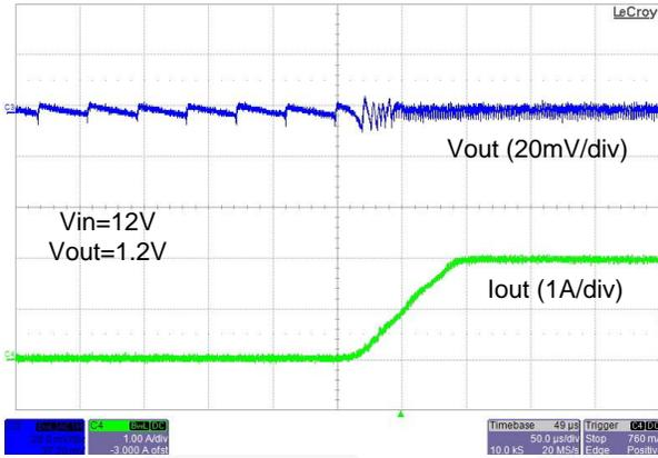
Figure 23. FAN2306A Transition from DCM to CCM
