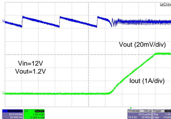
Figure 17. FAN2306MA Transition from DCM to CCM
