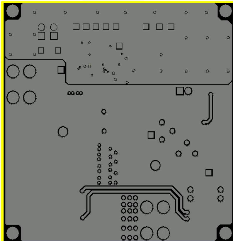
Figure 31. Evaluation Board Inner Layer 1 Copper
