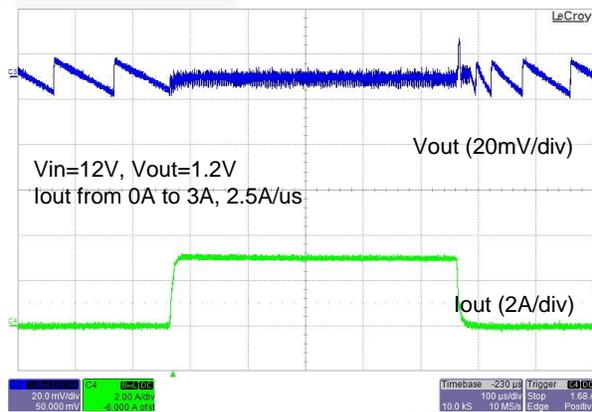
Figure 27. FAN2306MA Load Transient from 0% to 50% Load Current
