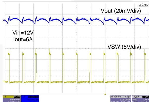
Figure 22. Static Output Ripple at Full Load
