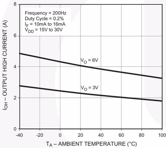
**Fig. 4 Output High Current vs. Ambient Temperature**
