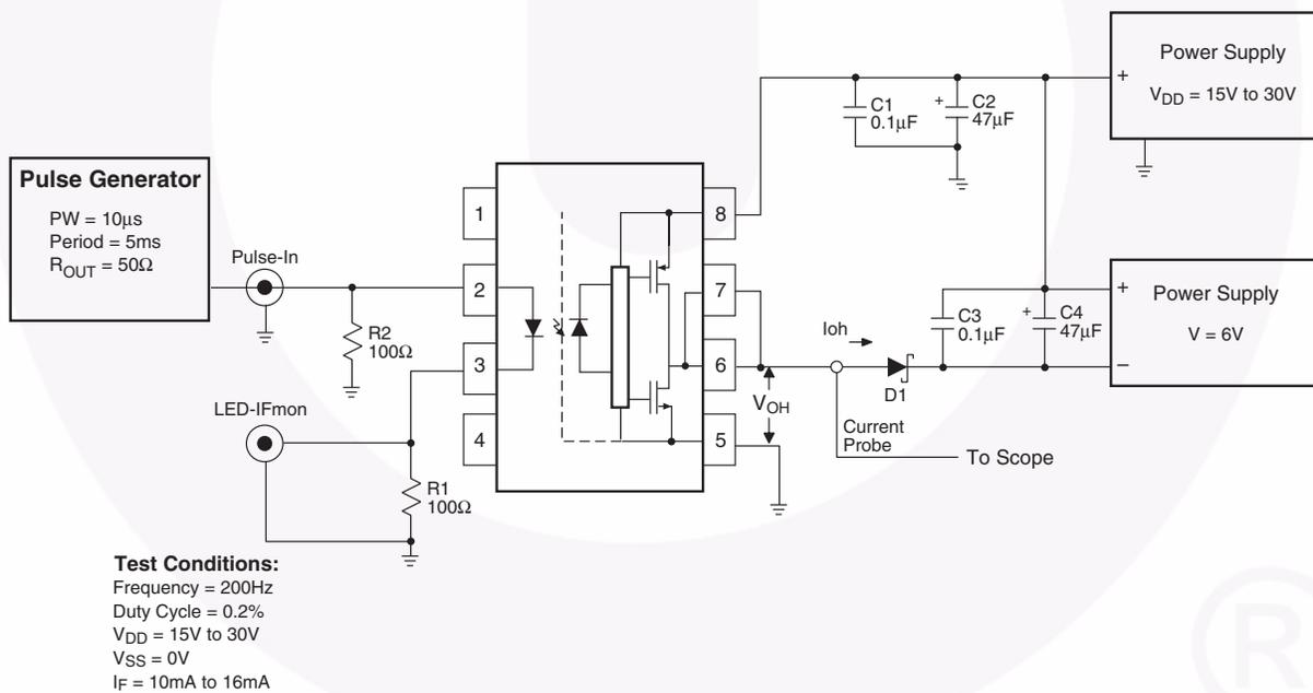
Figure 21. I<sub>OH</sub> Test Circuit
