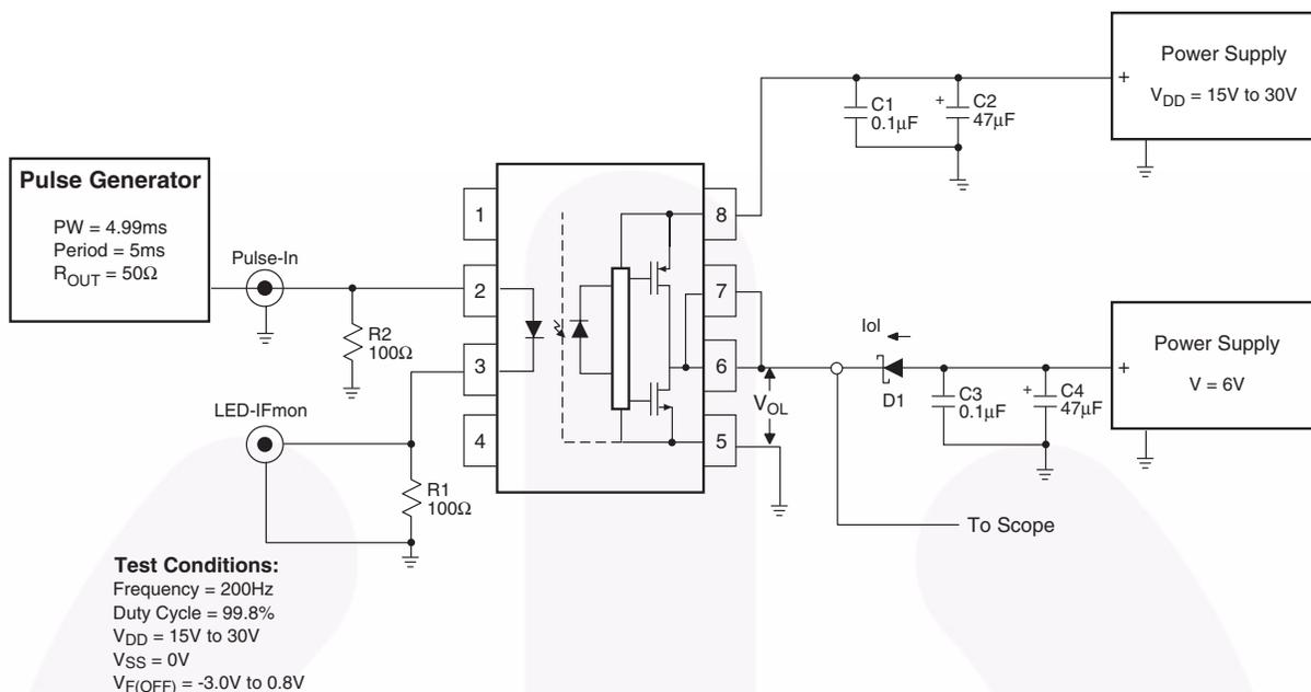
Figure 20. I<sub>OL</sub> Test Circuit
