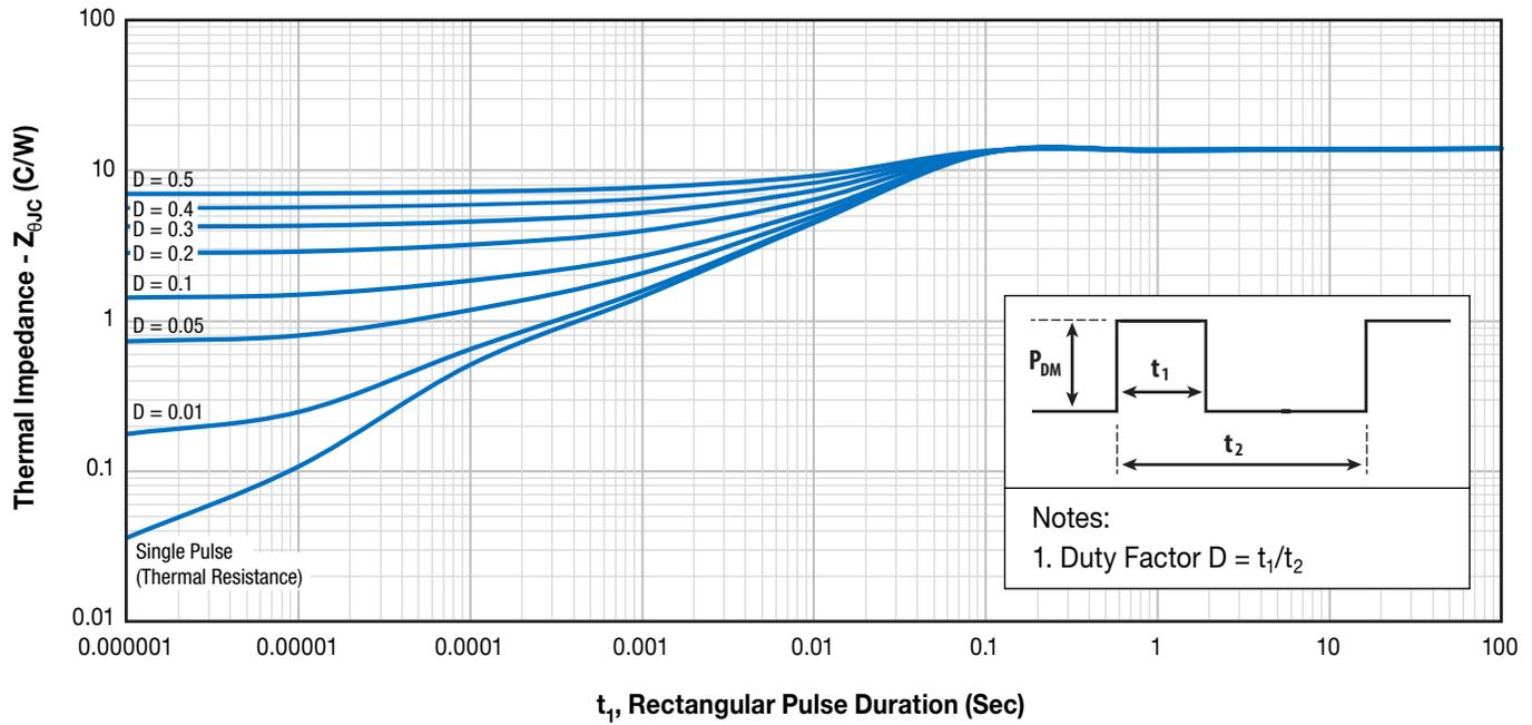
Figure 13. Transient Thermal Impedance, Junction to Case
