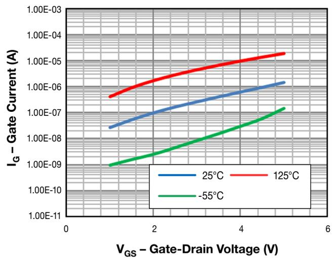
Figure 3. Gate-Source Leakage Current vs. Ambient Temperature
