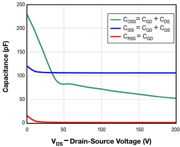
Figure 10. Typical Inter-Electrode Capacitance vs. Drain-Source Voltage
