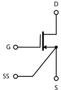
**NOTE:** SS pin is connected directly to source of internal die.
