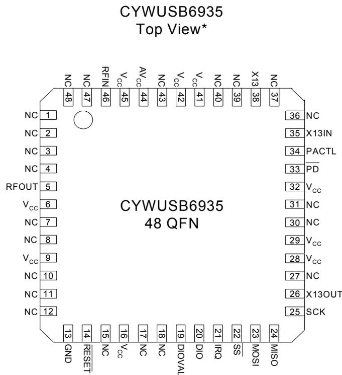
**Figure 8-2. CYWUSB6935, 48 QFN – Top View**
