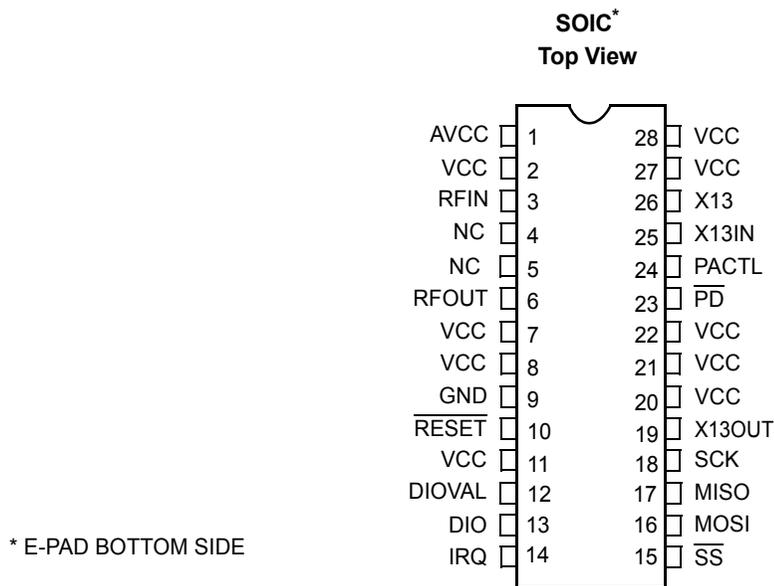
**Figure 8-1. CYWUSB6935, 28 SOIC – Top View**
