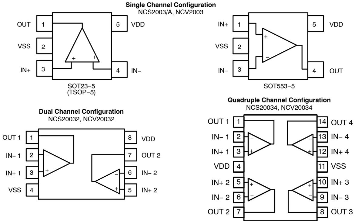
Figure 1. Pin Connections
