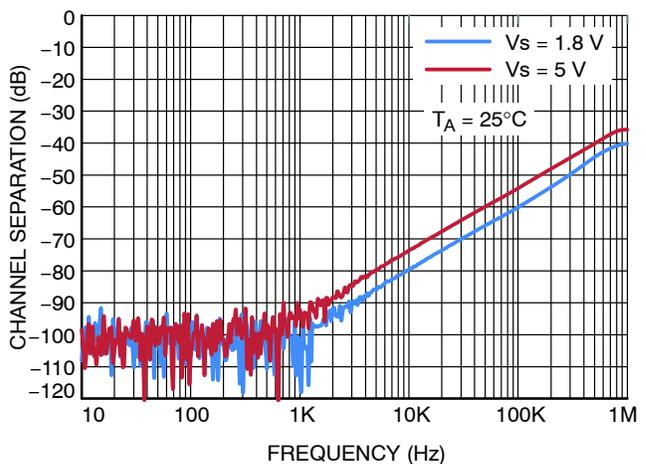
Figure 25. Channel Separation
