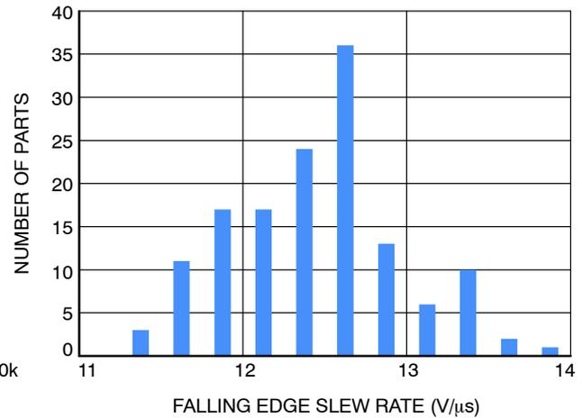
Figure 23. Falling Edge Slew Rate @  $V_S = 5\text{ V}$
