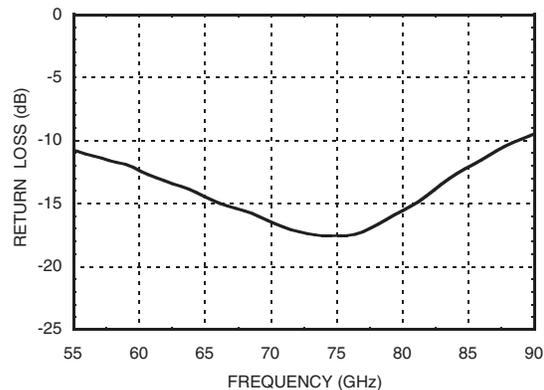
Note 1: Measured Performance Characteristics (Typical Performance at 25°C) Test data is taken with probes on RFIN and RFOUT1 with RFOUT2 left open.
