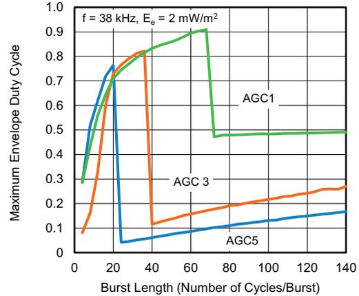
Fig. 8 - Maximum Envelope Duty Cycle vs. Burst Length
