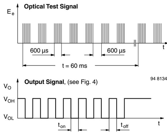
Fig. 3 - Test Signal
