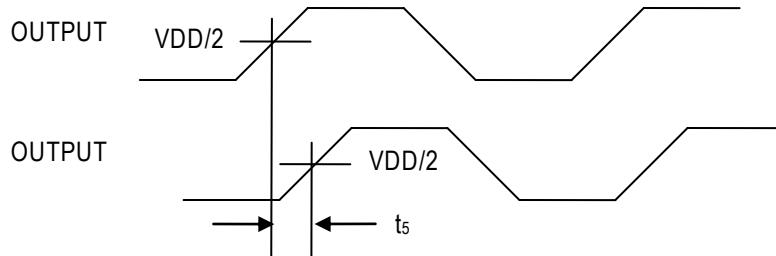
**Input-Output Propagation Delay**
