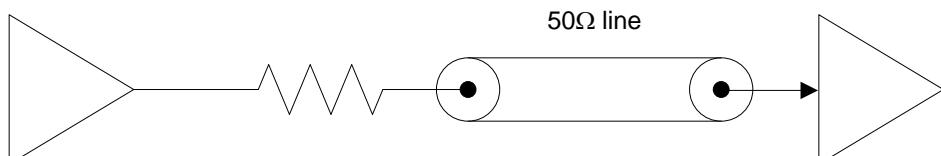
Connect a  $33\ \Omega$  series resistor at each of the output clocks to enhance the stability of the output signal
