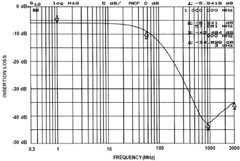
Figure 3. Attenuation Curve for CM1454 RC Filters: 1, 2, 6, 7, and 8
