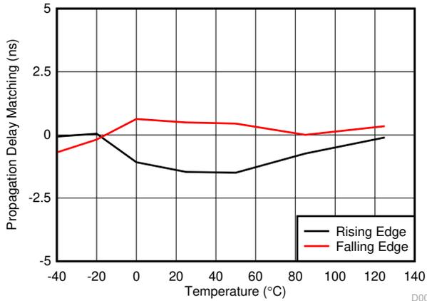
**Figure 7-16. Propagation Delay Matching ( $t_{DM}$ ) vs Temperature**
