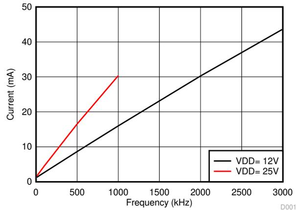
**Figure 7-5. Per Channel Current Consumption (I<sub>VDDA/B</sub>) vs Frequency (1-nF Load, VDD = 12 V or 25 V)**
