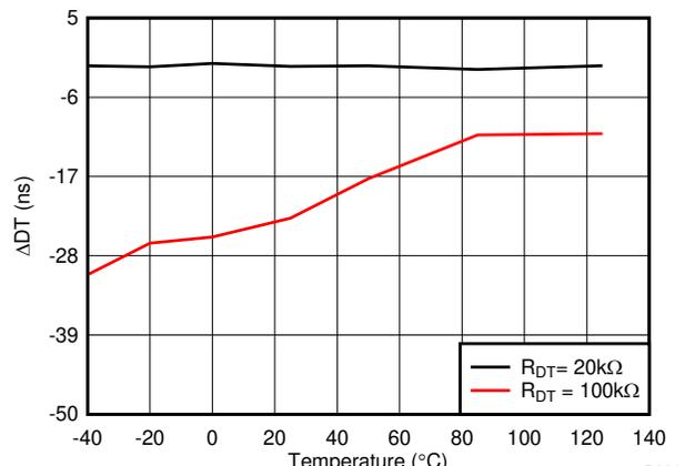
**Figure 7-25. Dead Time Matching vs Temperature (with R<sub>DT</sub> = 20 kΩ and 100 kΩ)**
