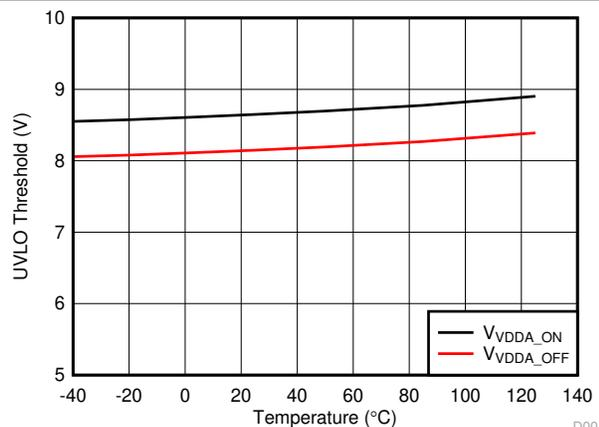
**Figure 7-20. VDD 8-V UVLO Threshold vs Temperature**
