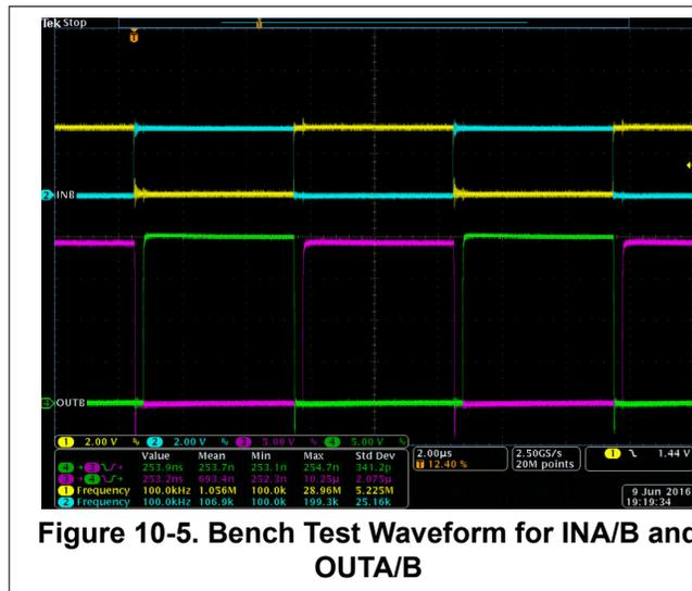
**Figure 10-5. Bench Test Waveform for INA/B and OUTA/B**
