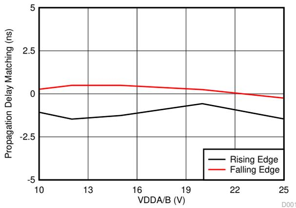
**Figure 7-15. Propagation Delay Matching (t<sub>DM</sub>) vs VDD**
