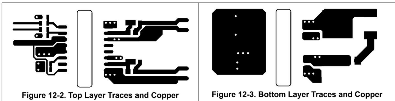
Figure 12-2. Top Layer Traces and Copper
