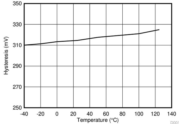
**Figure 7-17. VDD 5-V UVLO Hysteresis vs Temperature**
