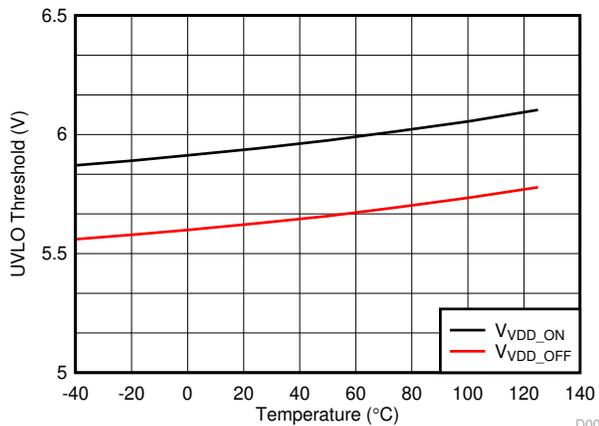
**Figure 7-18. VDD 5-V UVLO Threshold vs Temperature**
