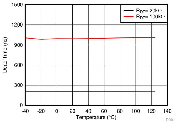
**Figure 7-24. Dead Time vs Temperature (with R<sub>DT</sub> = 20 kΩ and 100 kΩ)**
