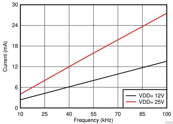
**Figure 7-6. Per Channel Current Consumption (I<sub>VDDA/B</sub>) vs Frequency (10-nF Load, VDD = 12 V or 25 V)**
