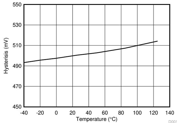
**Figure 7-19. VDD 8-V UVLO Hysteresis vs Temperature**
