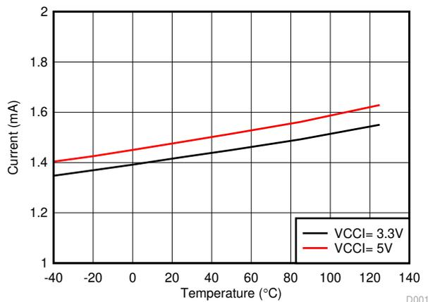
**Figure 7-9. I<sub>VCCI</sub> Quiescent Supply Current vs Temperature (No Load, Input Low, No Switching)**
