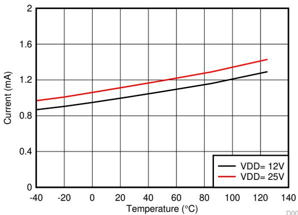
**Figure 7-8. Per Channel (I<sub>VDDA/B</sub>) Quiescent Supply Current vs Temperature (No Load, Input Low, No Switching)**
