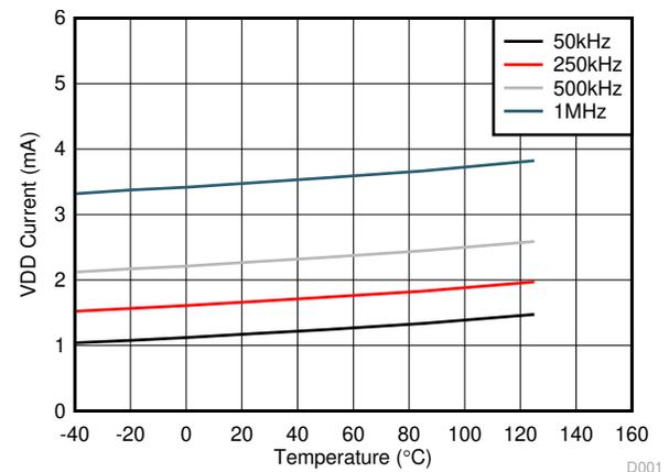
**Figure 7-7. Per Channel (I<sub>VDDA/B</sub>) Supply Current vs. Temperature (No Load, Different Switching Frequencies)**
