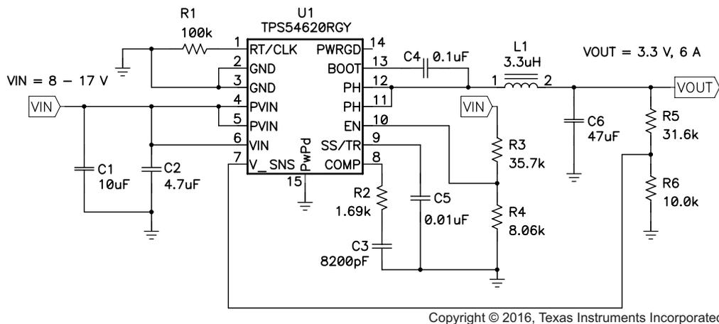
Figure 34. Typical Application Circuit
