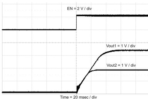
Figure 33. Simultaneous Start-Up
