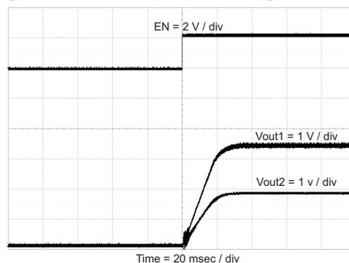
Figure 29. Ratiometric Start-Up Using Coupled SS/TR Pins
