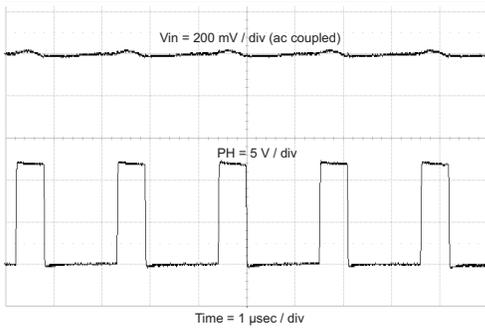
**Figure 45. Input Voltage Ripple With No Load**
