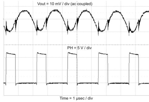
**Figure 44. Output Voltage Ripple With Full Load**
