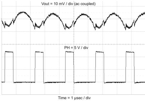
**Figure 43. Output Voltage Ripple With No Load**
