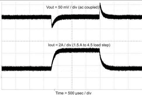
Figure 37. Load Transient
