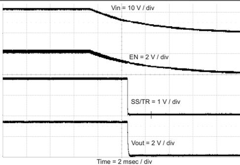
Figure 41. Shutdown With VIN
