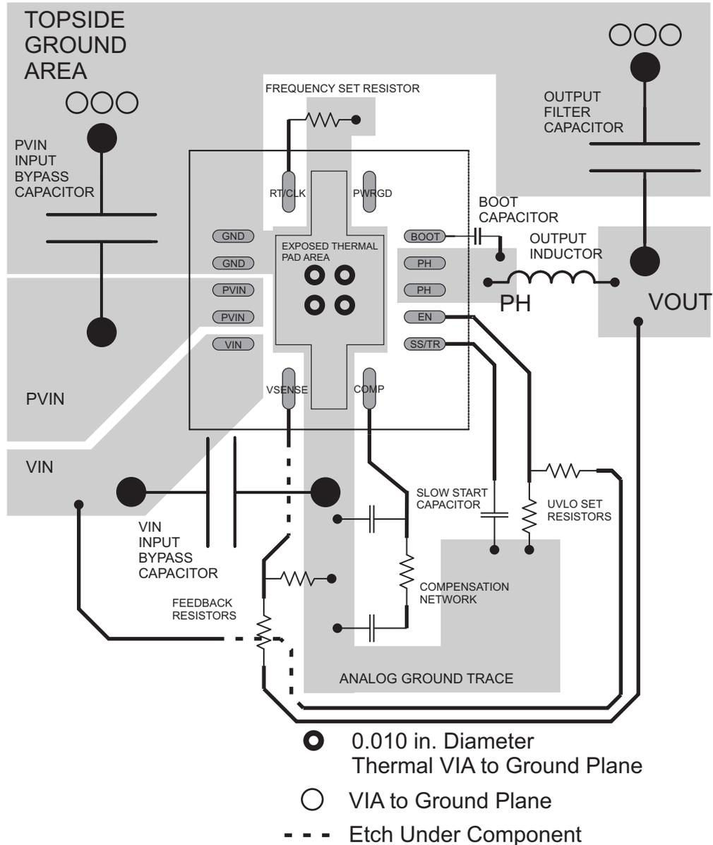
Figure 55. PCB Layout
