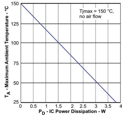
Figure 52. Maximum Ambient Temperature vs IC Power Dissipation
