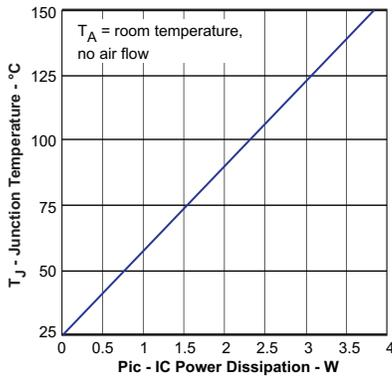
Figure 53. Junction Temperature vs IC Power Dissipation
