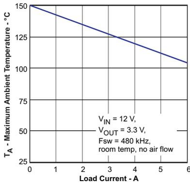
Figure 51. Maximum Ambient Temperature vs Load Current
