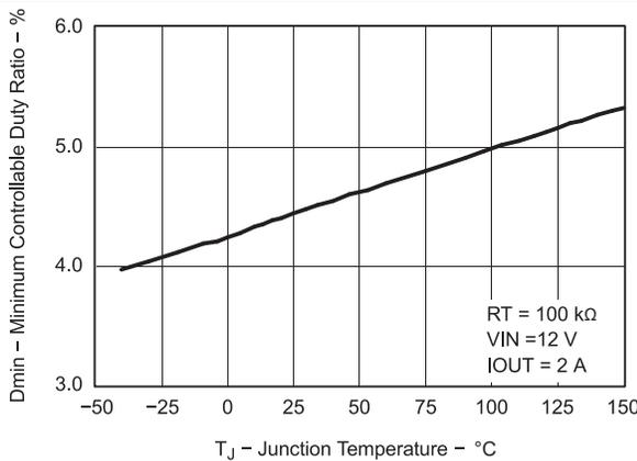
Figure 15. Minimum Controllable Duty Ratio vs Junction Temperature
