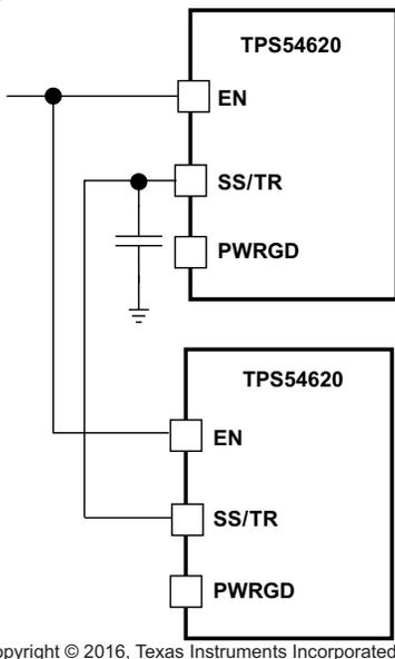
Figure 28. Ratiometric Start-Up Sequence
