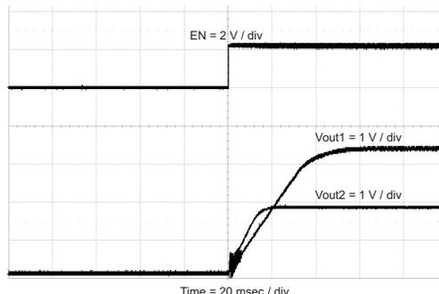
Figure 31. Ratiometric Start-Up With Vout1 Leading Vout2
