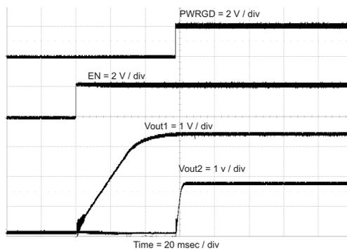
Figure 27. Sequential Start-Up Using EN and PWRGD
