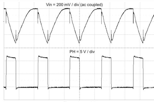
**Figure 46. Input Voltage Ripple With Full Load**
