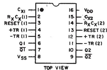
TERMINALS 1, 8, 15 ARE ELECTRICALLY CONNECTED INTERNALLY
