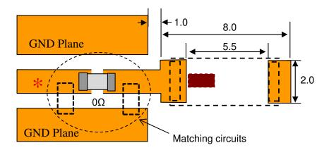
\* Line width should be designed to match 50ohm characteristic impedance, depending on your PCB material and thickness (distance to GND)
