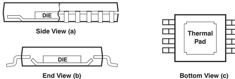
NOTE: The thermal pad is electrically isolated from all terminals in the package.
