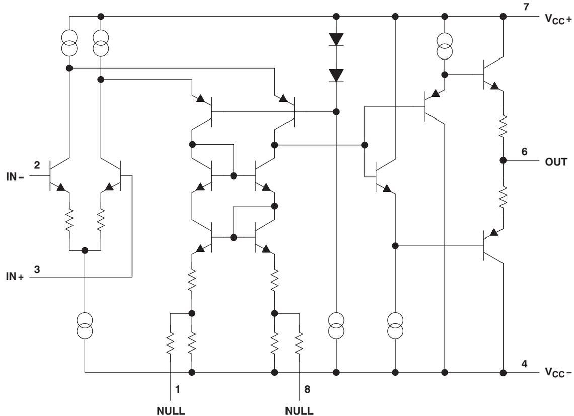
Pin numbers are for the D, DGN, and JG packages.
