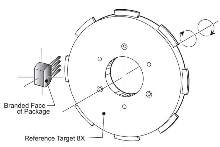
**Target Flux Density versus Target Rotation**
