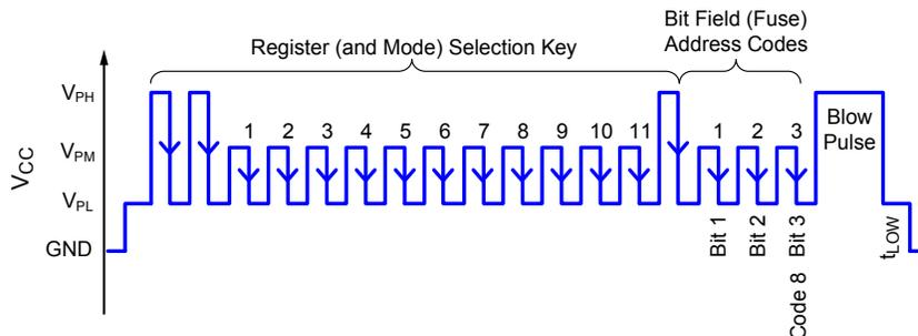
Figure 13. Example of Blow mode programming pulses applied to the VCC pin. In this example, the  $B_{OP}$  Magnitude Selection register (BOPSEL) is addressed to code 8 (bit 3, or 3  $V_{PM}$  pulses) and its value is permanently blown.
