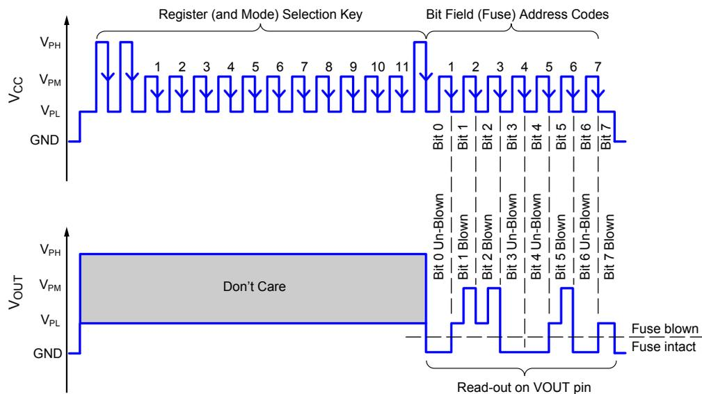
Figure 11. Read mode example. Pulse sequence for accessing the  $B_{OP}$  Selection register (BOPSEL) and reading back the status of each of the eight bit fields. In this example, the code (blown fuses) is  $2 + 2^2 + 2^5 + 2^7 = 166$  (10100110). After each address pulse is sent, the voltage on the VOUT pin will be at GND for un-blown fuses and at  $V_{CC}$  (at  $V_{PL}$  or  $V_{PM}$ ) for blown fuses.
