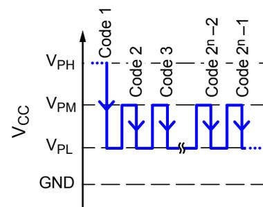
Figure 8. Try mode bit field addressing pulses.
