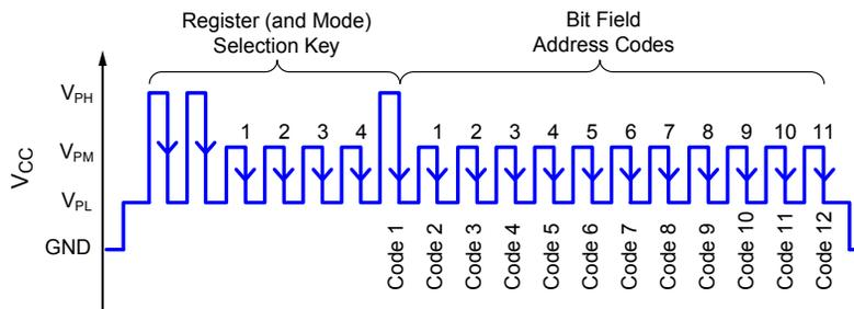
Figure 12. Example of Try mode programming pulses applied to the VCC pin. In this example,  $B_{OP}$  Positive Trim, Down-Counting register is addressed to code 12 by the eleven  $V_{PM}$  pulses (code 1 is selected automatically at the falling edge of the register-mode selection key).
