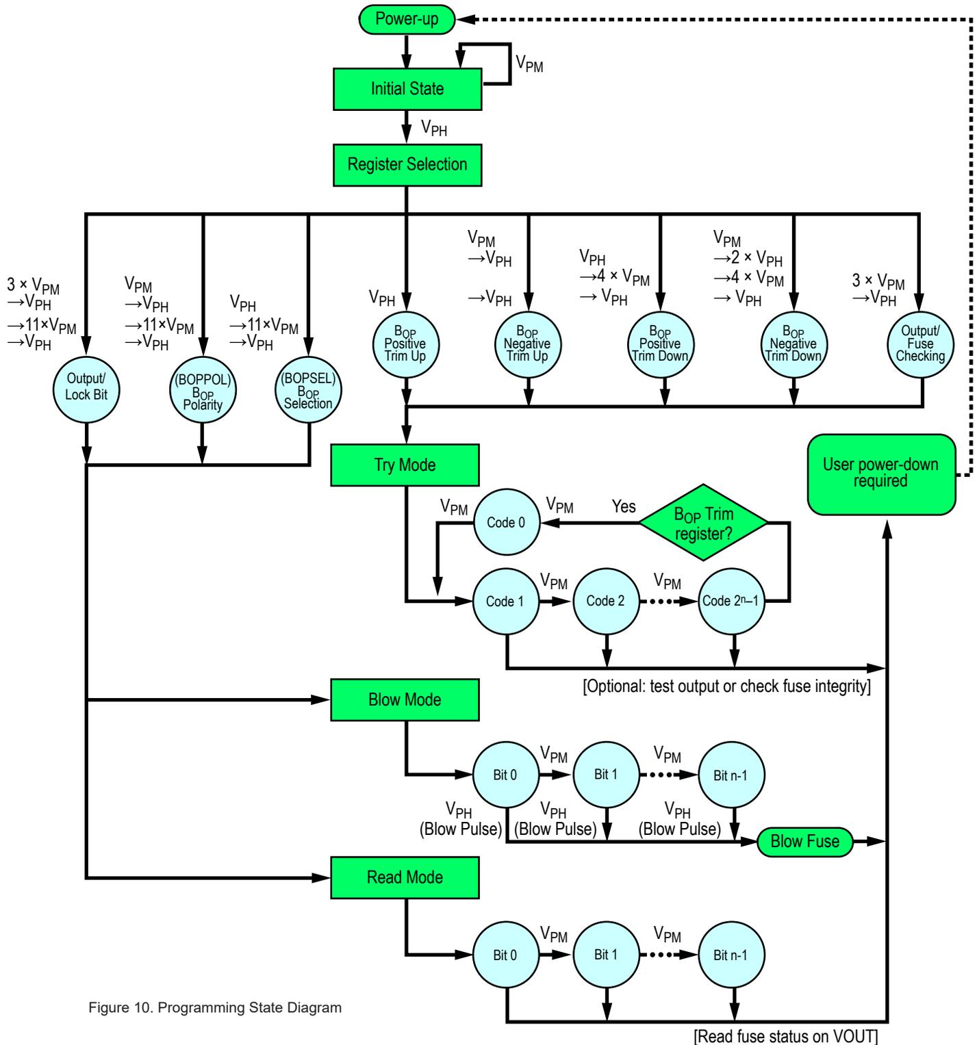
Figure 10. Programming State Diagram
