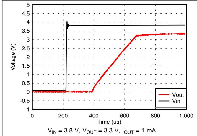
Figure 23.  $V_{IN}$  Power-Up
