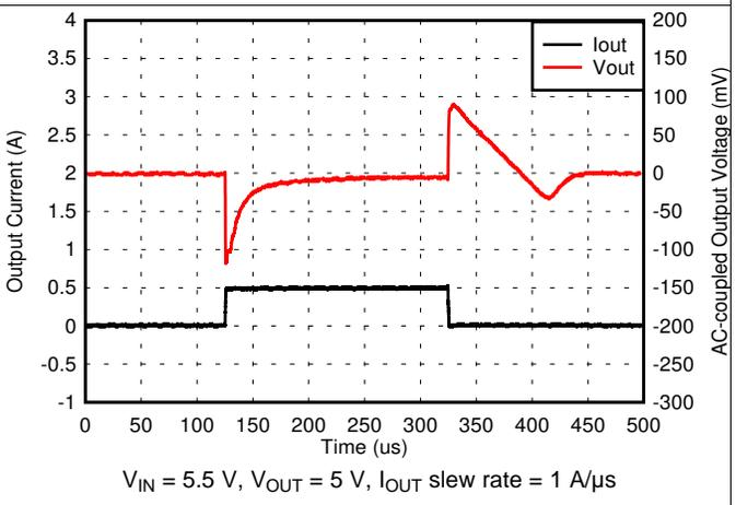
Figure 22. 5-V, 1-mA to 500-mA Load Transient
