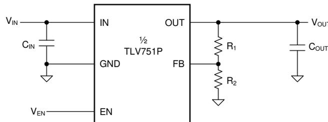
**Figure 38. Adjustable Operation**
