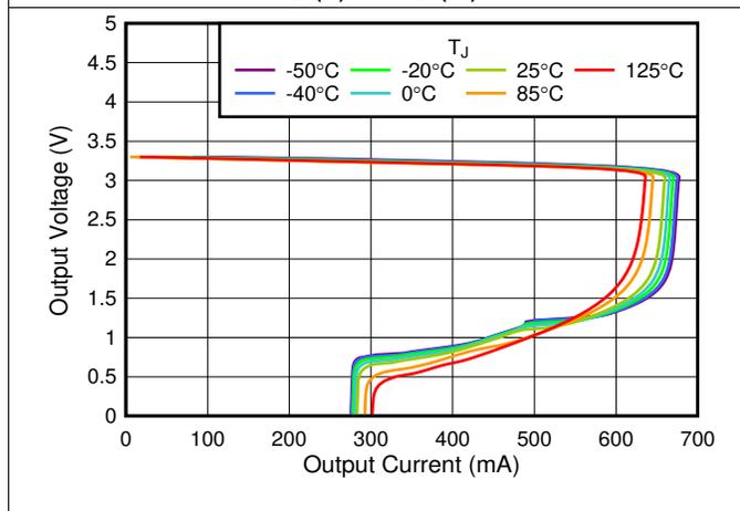
Figure 17. 3.3-V Foldback Current Limit vs  $I_{OUT}$
