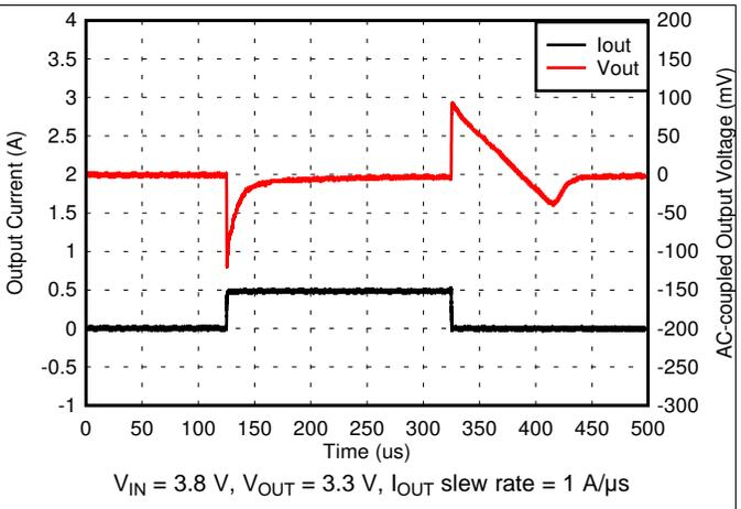
Figure 20. 3.3-V, 1-mA to 500-mA Load Transient
