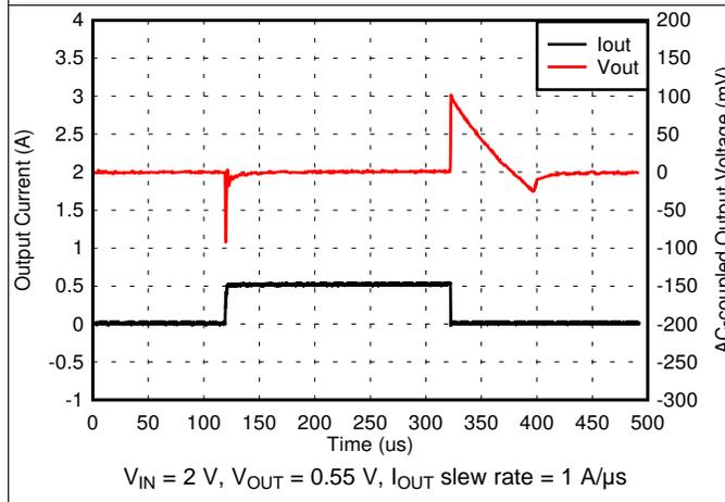
Figure 21. 0.55-V, 1-mA to 500-mA Load Transient
