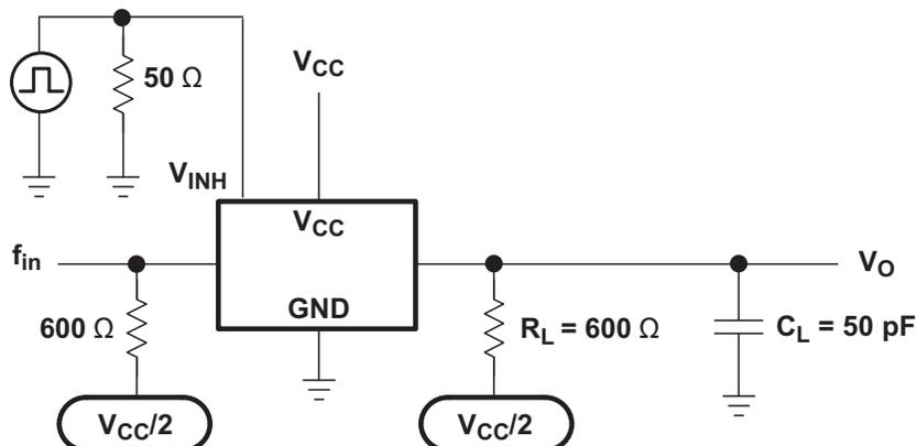
Figure 9. Crosstalk Between Control Input and Switch Output
