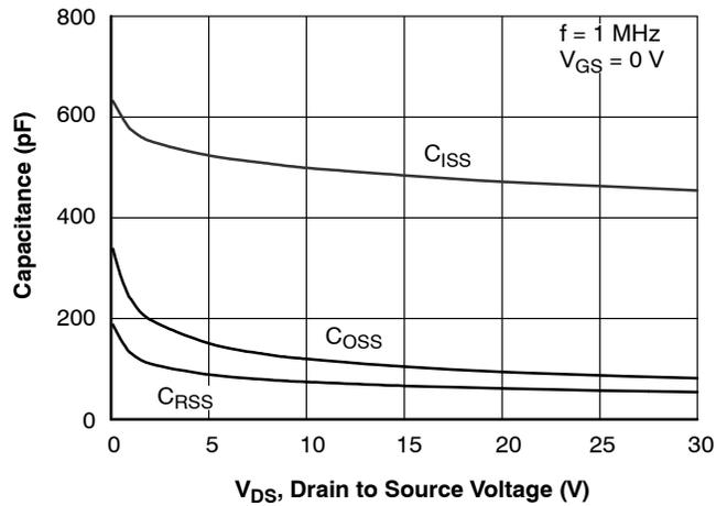
Figure 8. Capacitance Characteristics
