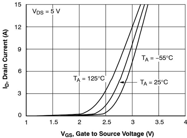
Figure 5. Transfer Characteristics
