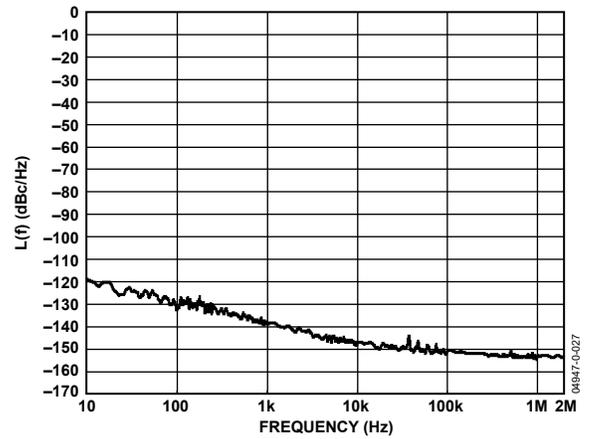
Figure 20. RF Divider and CML Driver Residual
