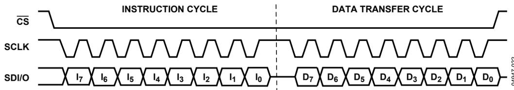
Figure 42. 2-Wire Serial Port Read Timing—Clock Stall High
