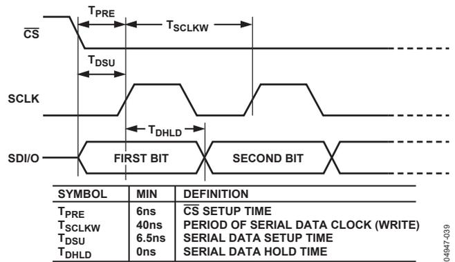
Figure 43. Timing Diagram for Data Write to AD9540
