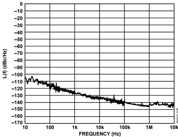
Figure 18. DDS/DAC Residual Phase Noise
