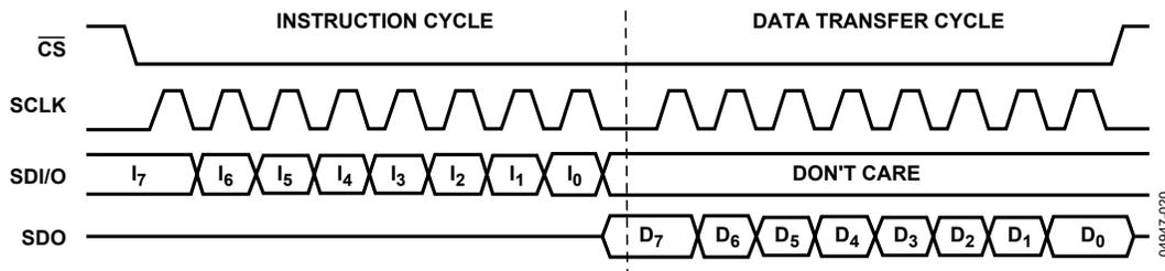
Figure 40. 3-Wire Serial Port Read Timing—Clock Stall Low
