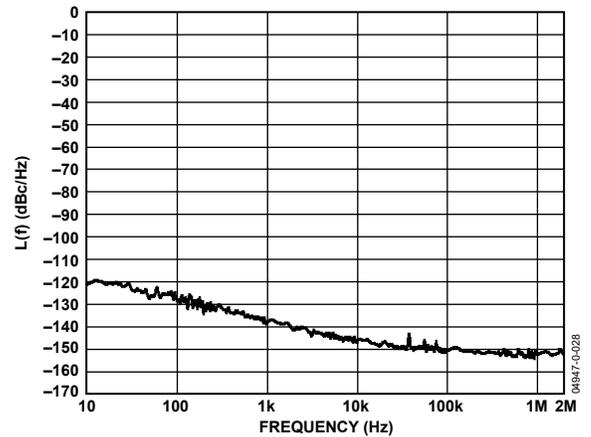
Figure 21. RF Divider and CML Driver Residual
