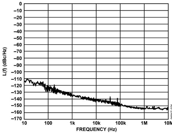
Figure 17. DDS/DAC Residual Phase Noise
