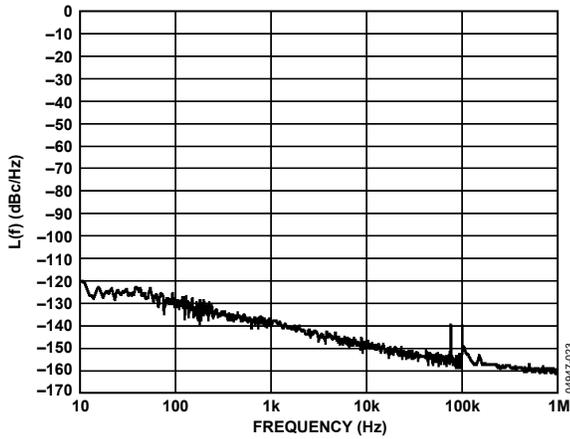
Figure 16. DDS/DAC Residual Phase Noise
