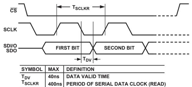
Figure 44. Timing Diagram for Data Read from AD9540
