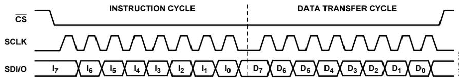
Figure 39. Serial Port Write Timing—Clock Stall Low
