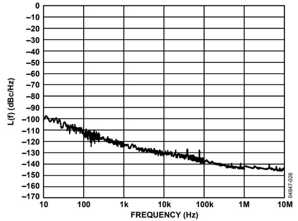
Figure 19. DDS/DAC Residual Phase Noise
