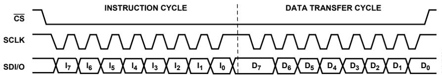
Figure 41. Serial Port Write Timing—Clock Stall High
