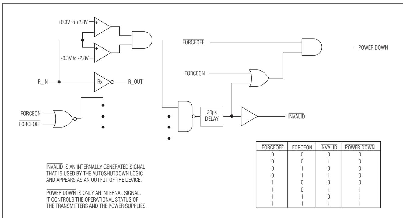
Figure 3. AutoShutdown Logic
