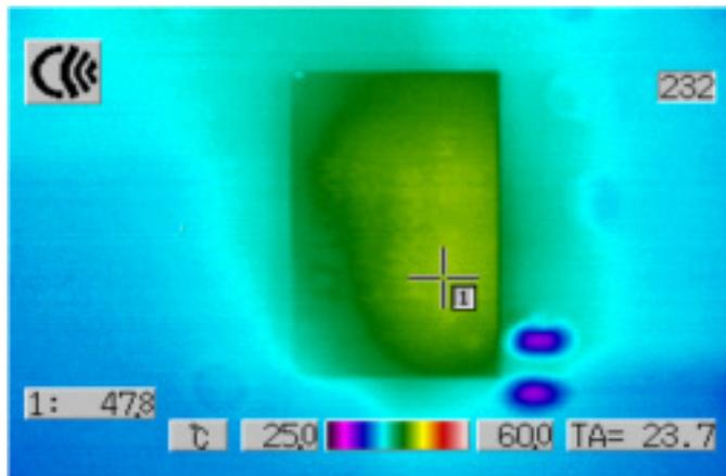
**Figure 16. Thermal Image 5V<sub>IN</sub> to 1.5V<sub>OUT</sub> at 10A
