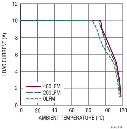
Figure 14. No Heat Sink with 5V<sub>IN</sub> to 2.5V<sub>OUT</sub>
