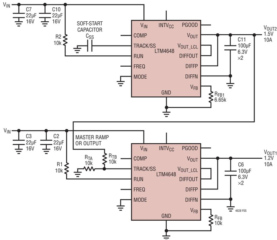
Figure 5. Dual Outputs (1.5V and 1.2V) with Tracking
