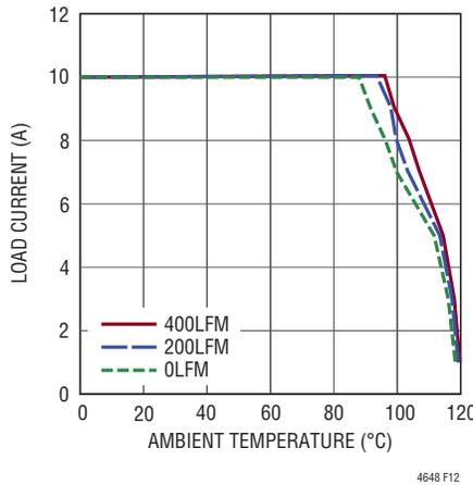
Figure 12. No Heat Sink with 5V<sub>IN</sub> to 1.5V<sub>OUT</sub>
