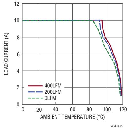
Figure 15. No Heat Sink with 5V<sub>IN</sub> to 3.3V<sub>OUT</sub>
