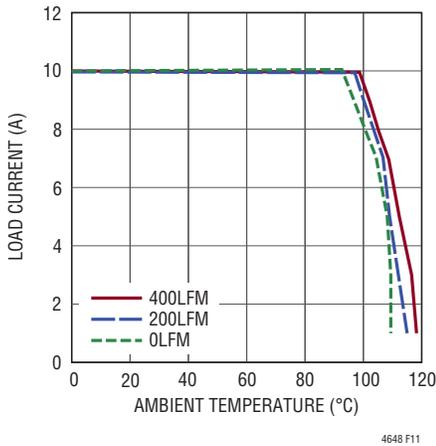
Figure 11. No Heat Sink with 3.3V<sub>IN</sub> to 1.5V<sub>OUT</sub>
