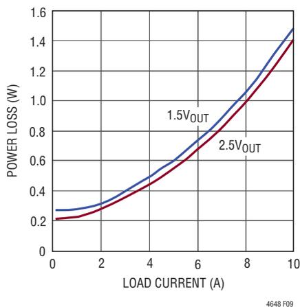
Figure 9. 3.3V<sub>IN</sub> to 2.5V<sub>OUT</sub> and 1.5V<sub>OUT</sub> Power Loss
