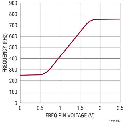
Figure 2. Operating Frequency vs FREQ Pin Voltage
