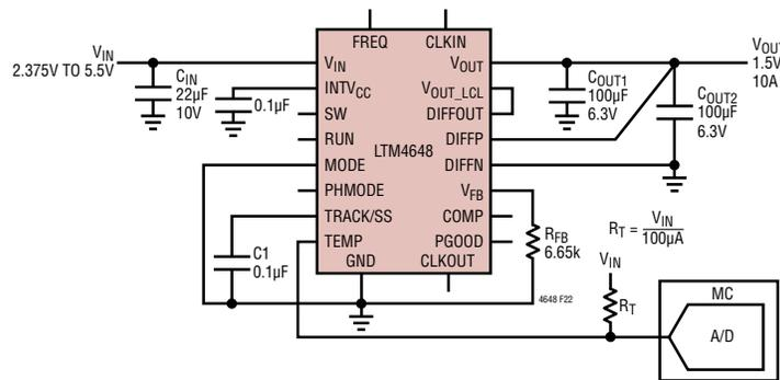
Figure 22. Single LTM4648 10A Design with Temperature Monitoring
