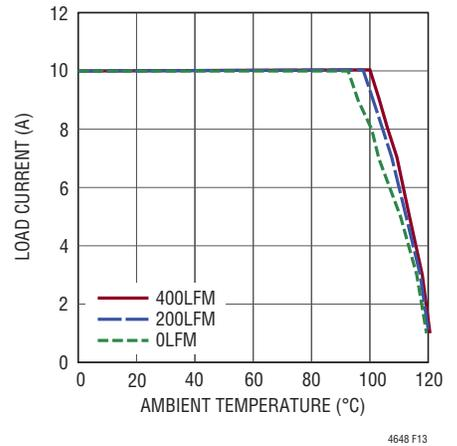
Figure 13. No Heat Sink with 3.3V<sub>IN</sub> to 2.5V<sub>OUT</sub>
