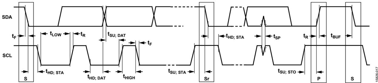
Figure 64. I<sup>2</sup>C Serial Port Timing
