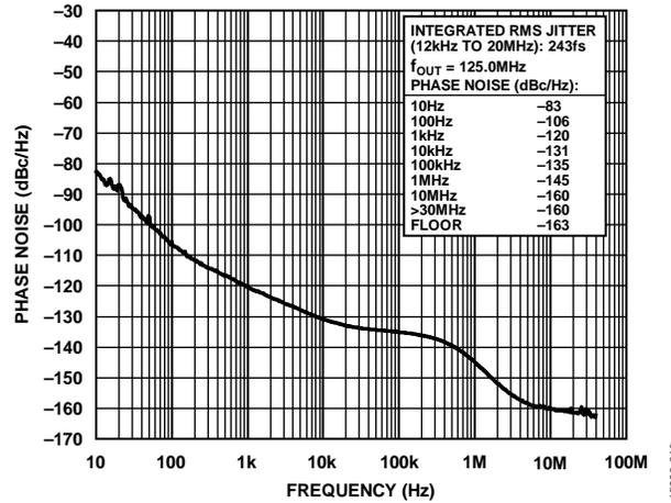
Figure 12. Absolute Phase Noise (PLL1, Configuration 4, HCSL Mode,  $f_{REF} = 125\text{ MHz}$ ,  $f_{OUT} = 125\text{ MHz}$ ,  $f_{COMP} = 19.2\text{ MHz}$  TCXO,  $f_{SYS} = 52\text{ MHz}$  Crystal, 0.1 Hz DPLL BW, Phase Buildout Mode)
