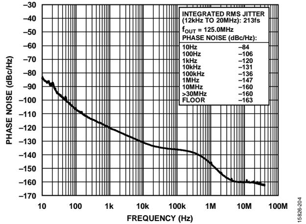
Figure 6. Absolute Phase Noise (PLL0, Configuration 4, HCSSL Mode,  $f_{REF} = 125\text{ MHz}$ ,  $f_{OUT} = 125.0\text{ MHz}$ ,  $f_{COMP} = 19.2\text{ MHz}$  TCXO,  $f_{SYS} = 52\text{ MHz}$  Crystal, 0.1 Hz DPLL BW, Phase Buildout Mode)
