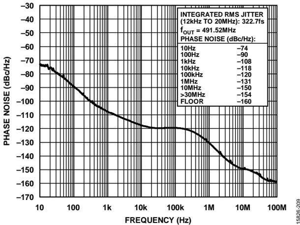
Figure 11. Absolute Phase Noise (PLL1, Configuration 3, HCSL Mode,  $f_{REF} = 1\text{ Hz}$ ,  $f_{OUT} = 491.52\text{ MHz}$ ,  $f_{COMP} = 19.2\text{ MHz}$  TCXO,  $f_{SYS} = 52\text{ MHz}$  Crystal, 50 MHz DPLL BW)
