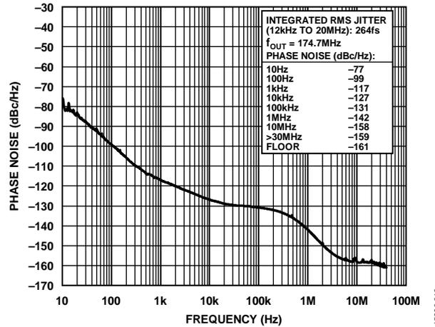
Figure 14. Absolute Phase Noise (PLL1, Configuration 6, HCSL Mode,  $f_{REF} = 155.52\text{ MHz}$ ,  $f_{OUT} = 174.7\text{ MHz}$ ,  $f_{SYS} = 52\text{ MHz}$  Crystal, 50 Hz DPLL BW, Phase Buildout Mode)
