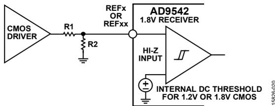
Figure 25. Single-Ended DC-Coupled Mode, 1.2 V or 1.8 V CMOS
