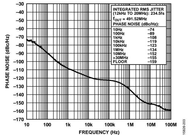
Figure 5. Absolute Phase Noise (PLL0, Configuration 3, HCSSL Mode,  $f_{REF} = 1\text{ Hz}$ ,  $f_{OUT} = 491.52\text{ MHz}$ ,  $f_{COMP} = 19.2\text{ MHz}$  TCXO,  $f_{SYS} = 52\text{ MHz}$  Crystal, 50 MHz DPLL BW)
