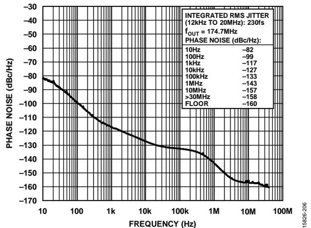
Figure 8. Absolute Phase Noise (PLL0, Configuration 6, HCSSL Mode,  $f_{REF} = 155.52\text{ MHz}$ ,  $f_{OUT} = 174.7\text{ MHz}$ ,  $f_{SYS} = 52\text{ MHz}$  Crystal, 50 Hz DPLL BW, Phase Buildout Mode)
