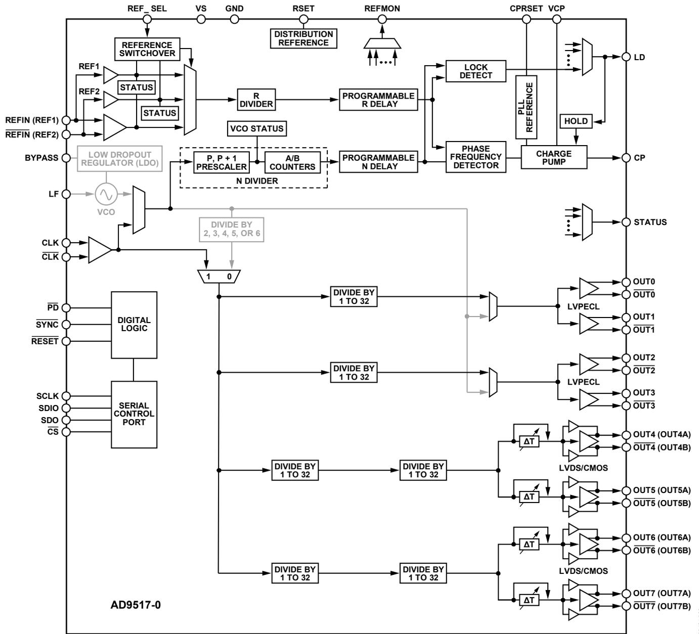
Figure 45. Clock Distribution or External VCO < 1600 MHz
