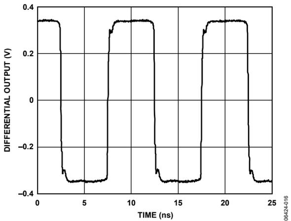
Figure 21. LVDS Output (Differential) at 100 MHz
