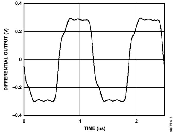
Figure 22. LVDS Output (Differential) at 800 MHz
