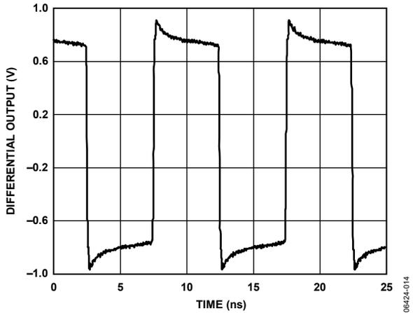
Figure 19. LVPECL Output (Differential) at 100 MHz
