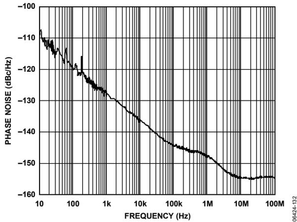
Figure 37. Phase Noise (Additive) CMOS at 250 MHz, Divide-by-4
