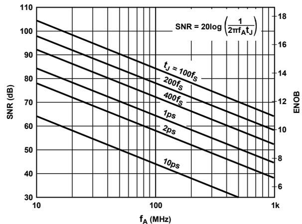
Figure 70. SNR and ENOB vs. Analog Input Frequency
