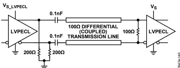
Figure 73. AC-Coupled LVPECL with Parallel Transmission Line
