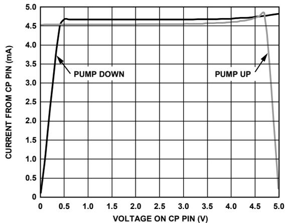
Figure 12. Charge Pump Characteristics at  $V_{CP} = 5.0 V$
