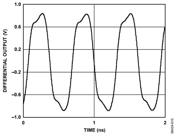
Figure 20. LVPECL Output (Differential) at 1600 MHz
