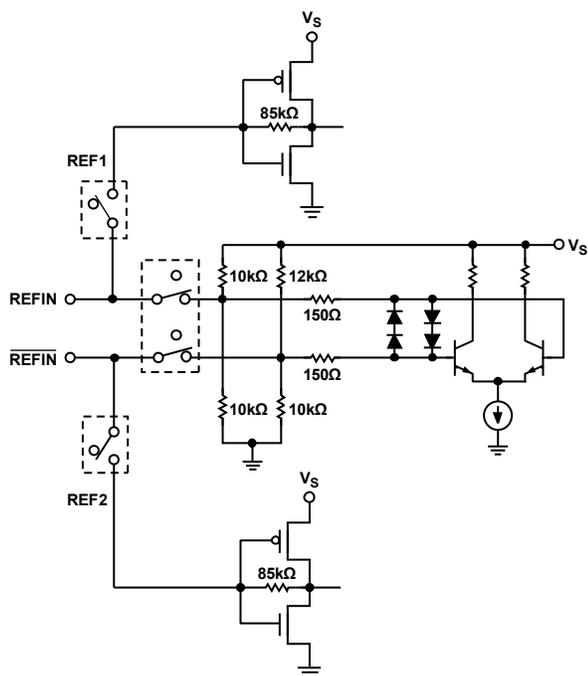
Figure 49. REF $\overline{\text{IN}}$  Equivalent Circuit
