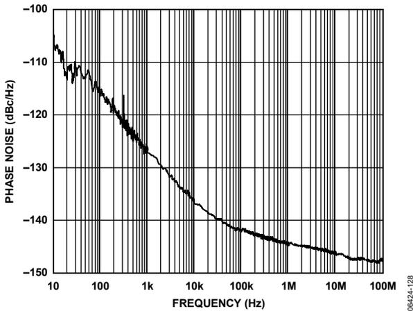
Figure 33. Phase Noise (Additive) LVPECL at 1600 MHz, Divide-by-1
