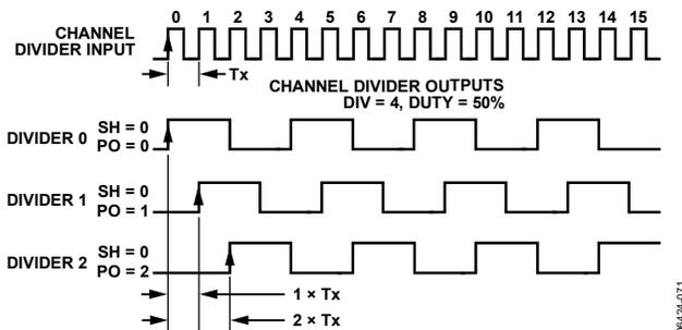
Figure 55. Effect of Coarse Phase Offset (or Delay)
