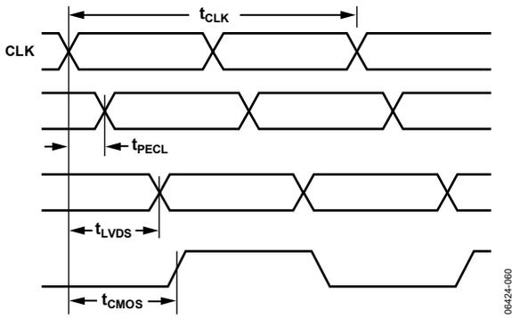
Figure 2. CLK/ $\overline{\text{CLK}}$  to Clock Output Timing, DIV = 1
