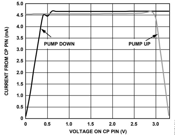
Figure 11. Charge Pump Characteristics at  $V_{CP} = 3.3 V$
