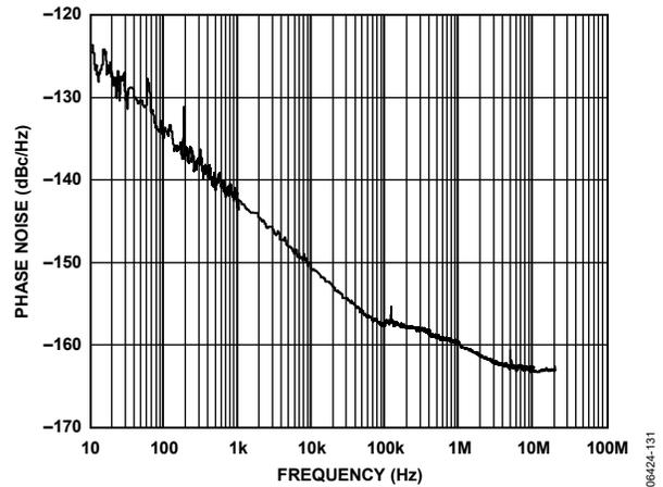
Figure 36. Phase Noise (Additive) CMOS at 50 MHz, Divide-by-20
