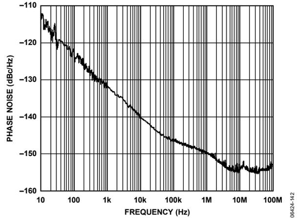
Figure 34. Phase Noise (Additive) LVDS at 200 MHz, Divide-by-1
