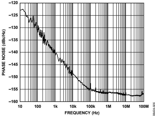
Figure 31. Phase Noise (Additive) LVPECL at 245.76 MHz, Divide-by-1
