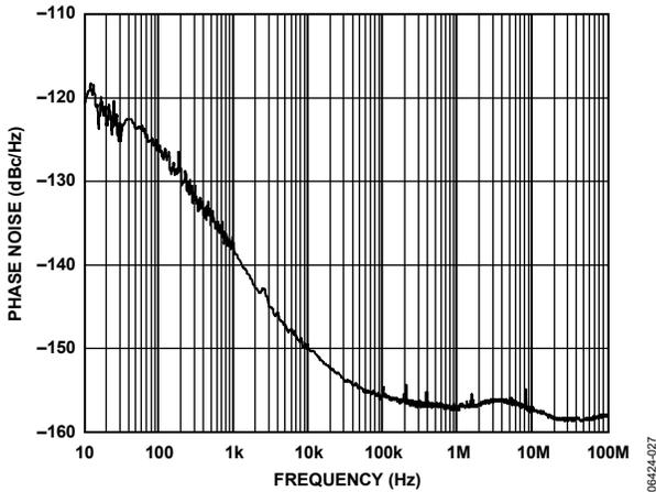
Figure 32. Phase Noise (Additive) LVPECL at 200 MHz, Divide-by-2
