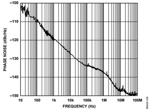
Figure 35. Phase Noise (Additive) LVDS at 800 MHz, Divide-by-2
