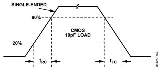
Figure 5. CMOS Timing, Single-Ended, 10 pF Load
