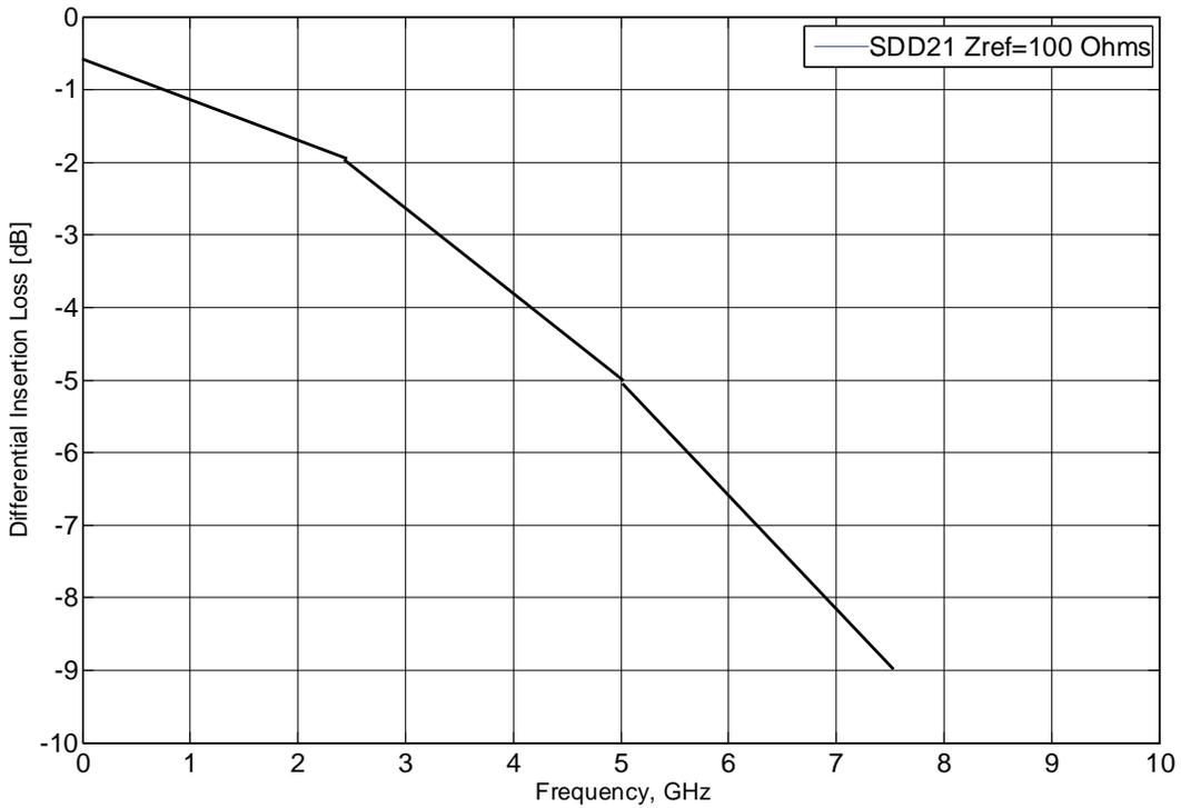
**Figure 1: Illustration of differential insertion loss requirement.**
