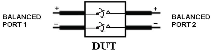
Differential Off Isolation Test Circuit
