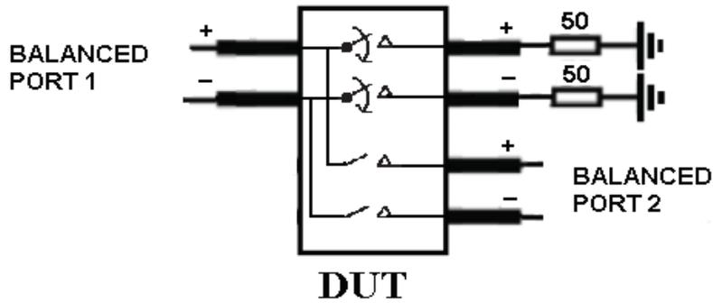
Differential Near End Crosstalk Test Circuit
