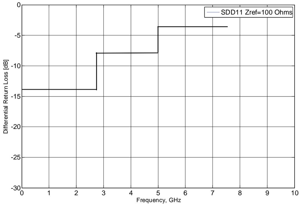
**Figure 2: Illustration of differential return loss requirement.**
