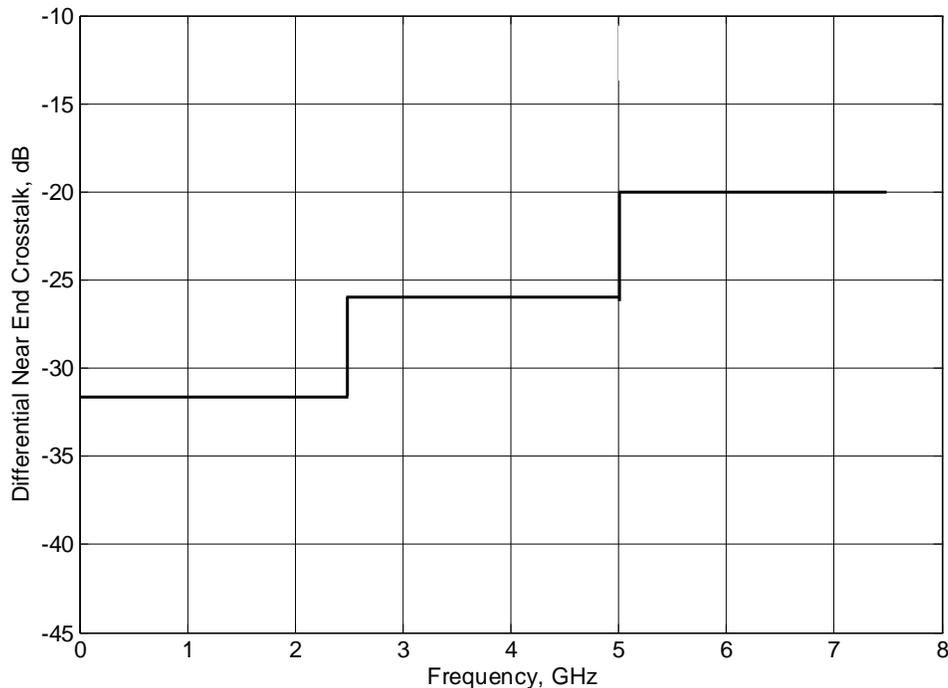
**Figure 3: Illustration of differential near end crosstalk requirement.**
