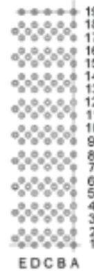
Recommended PCB hole mounting pattern for row differential applications
