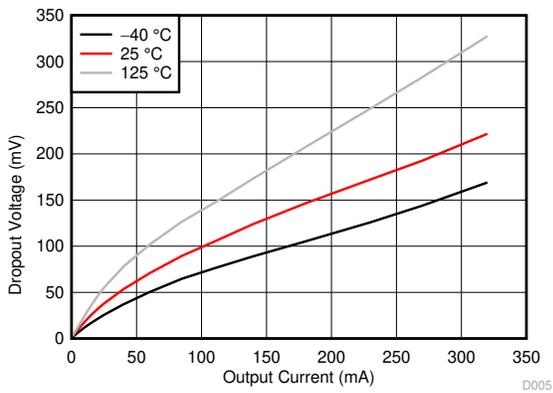
Figure 6-5. Dropout Voltage vs Output Current
