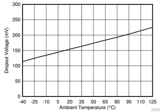
Figure 6-6. Dropout Voltage vs Ambient Temperature
