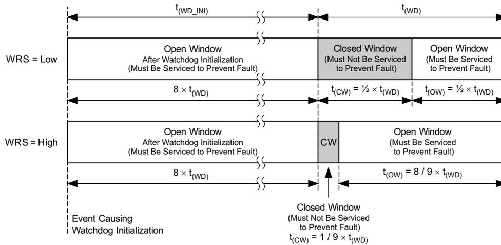
**Figure 7-3. Watchdog Initialization, Open Window and Closed Window**
