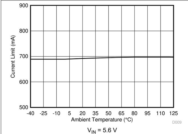
**Figure 6-9. Output Current Limit ( $I_{LIM}$ ) vs Ambient Temperature**
