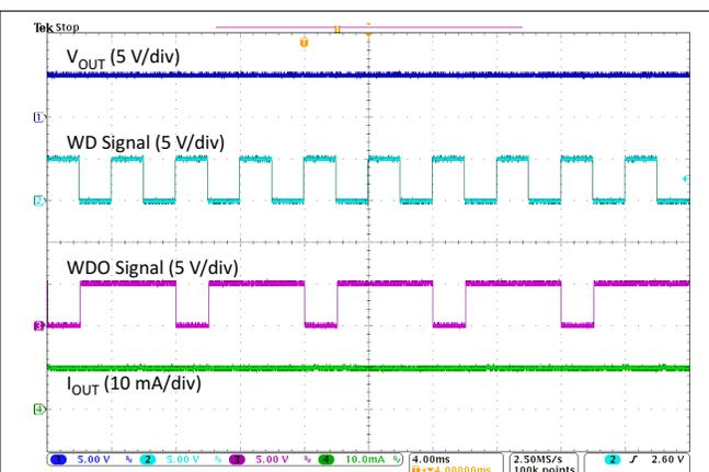
**Figure 8-3. TPS7B6350-Q1 Watchdog Fault (High-Frequency Watchdog Service Signal)**
