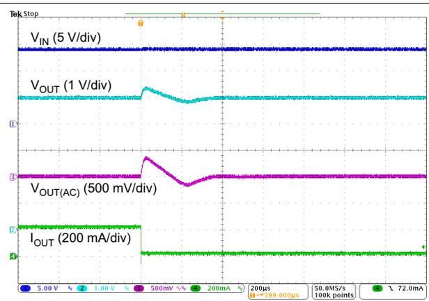
$V_{OUT} = 5\text{ V}$ ,  $C_{OUT} = 10\text{ }\mu\text{F}$ ,  $I_{OUT} = 200\text{ mA}$  to  $1\text{ mA}$
