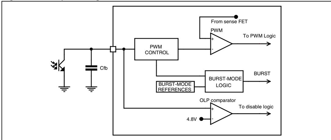
Figure 35. FB pin configuration
