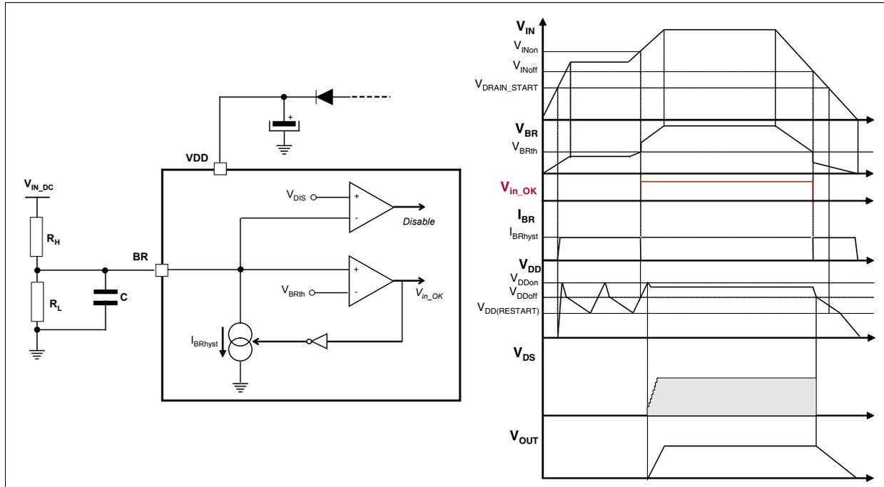
Fixed the  $V_{INon}$  and the  $V_{INoff}$  levels, with reference to [Figure 38](#), the following relationships can be established for the calculation of the resistors  $R_H$  and  $R_L$ :
