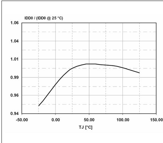
**Figure 14. Operating supply current (switching) vs  $T_J$**
