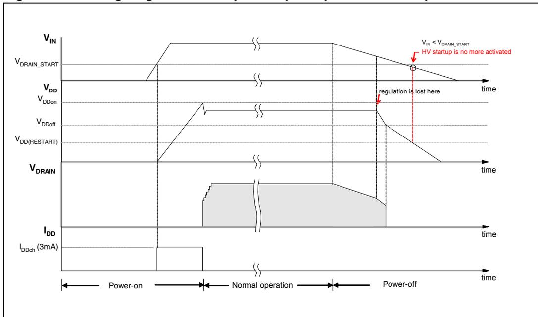
Figure 24. Timing diagram: Start-up phase and soft start (case 1)
