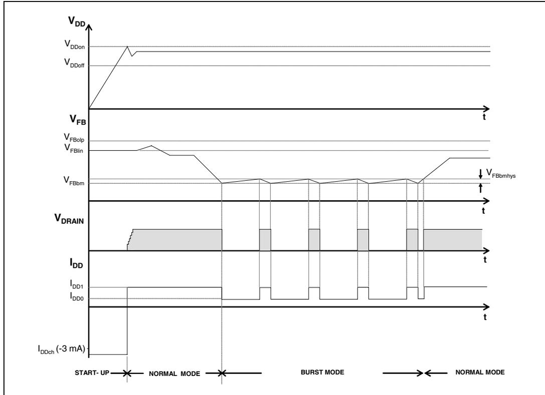
Figure 23. Timing diagram: normal power-up and power-down sequences
