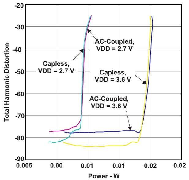
Figure 6. Headphone Power vs THD, 32 Ω Load
