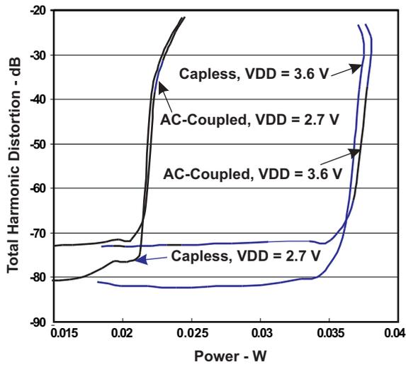
Figure 5. Headphone Power vs THD, 16 Ω Load
