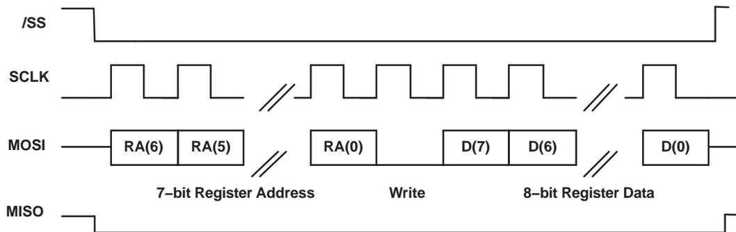
Figure 15. SPI Write
