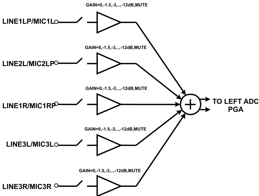
Figure 32. Left Channel Single-Ended Analog Input Mixing Configuration
