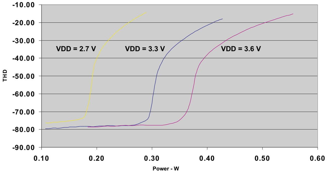
Figure 9. Speaker Power vs THD, 8 Ω Load
