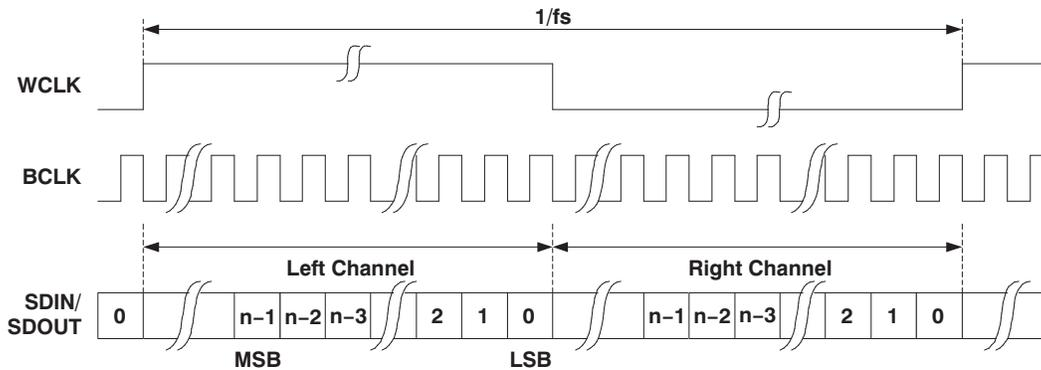
Figure 22. Right Justified Serial Bus Mode Operation
