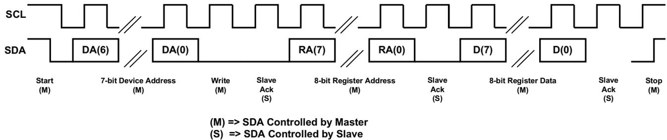
Figure 18. I<sup>2</sup>C Write
