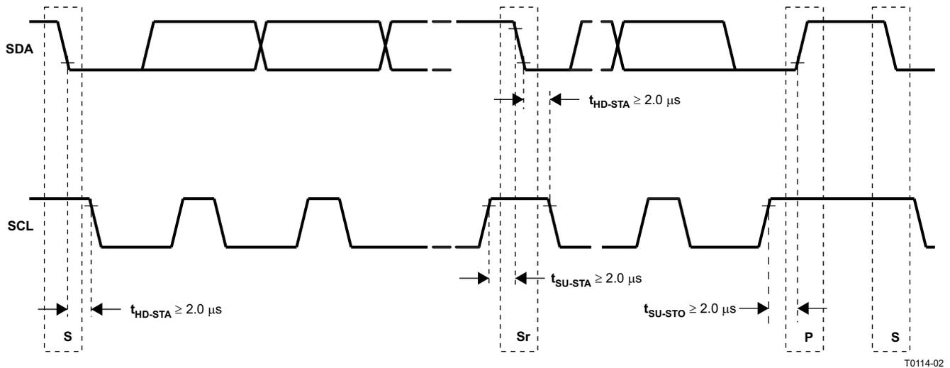
Figure 17. I<sup>2</sup>C Interface Timing
