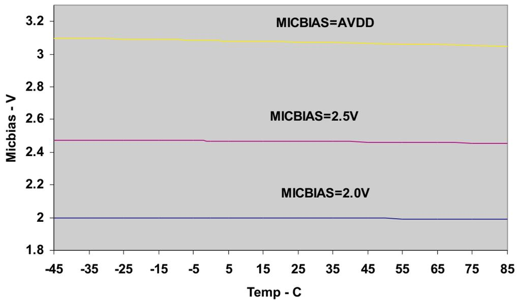
Figure 13. MICBIAS Output Voltage vs Ambient Temperature
