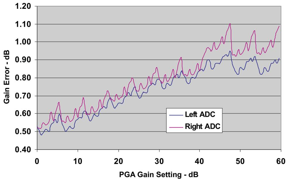
Figure 11. ADC Gain Error vs PGA Gain Setting
