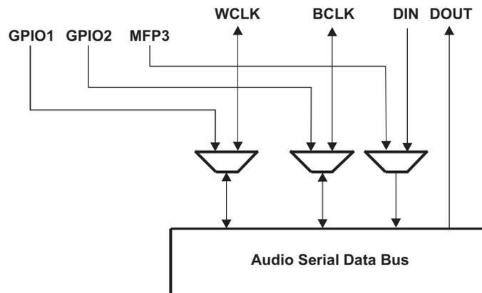
**Figure 20. Alternate Audio Bus Multiplexing Function**
