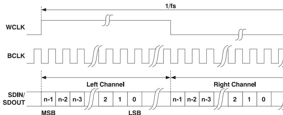
Figure 23. Left Justified Serial Data Bus Mode Operation
