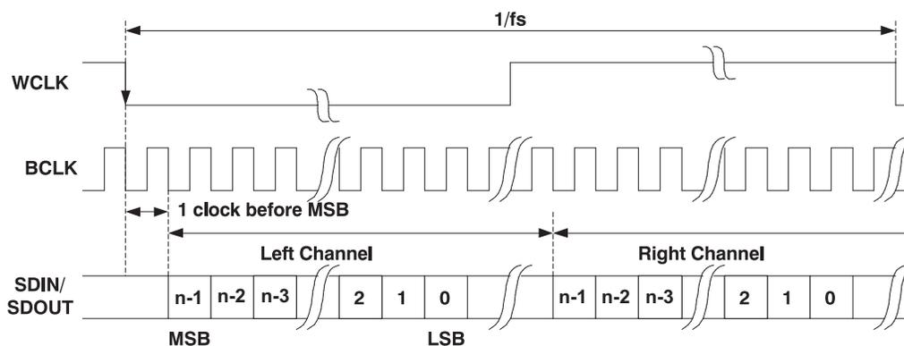
Figure 24. I<sup>2</sup>S Serial Data Bus Mode Operation
