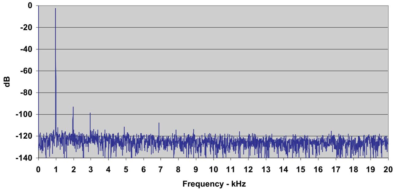
Figure 8. Line Input to ADC FFT Plot
