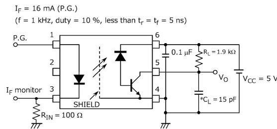
\* $C_L$  is approximately 15 pF which includes probe and stray wiring capacitance.
