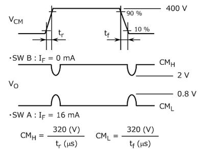
Fig. 13.1.6 Common-Mode Transient Immunity Test Circuit and Waveform
