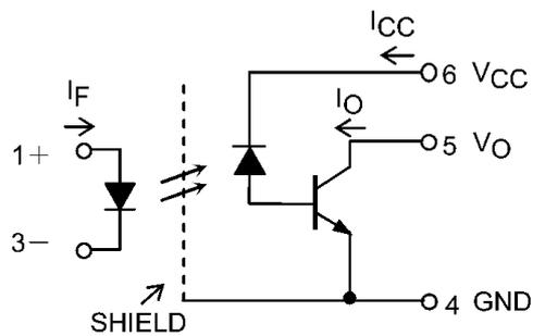
Note: A 0.1- $\mu$ F bypass capacitor must be connected between pin 6 and pin 4.
