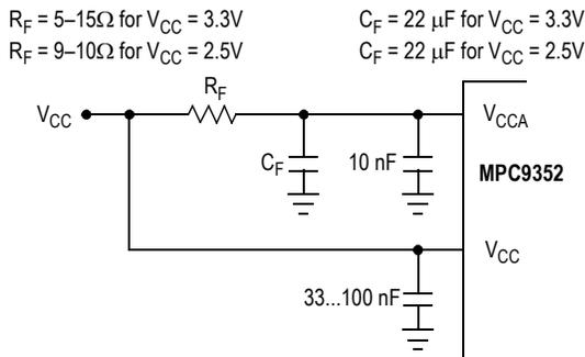
Figure 7.  $V_{CCA}$  Power Supply Filter
